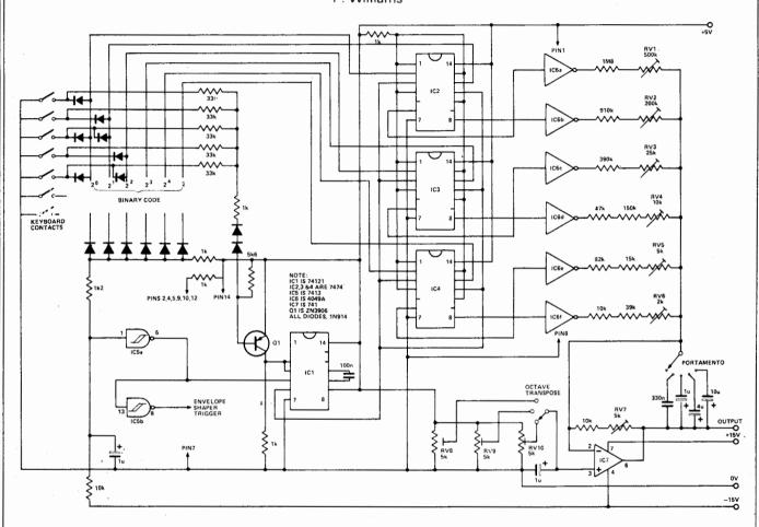
This circuit was designed to overcome all the problems associated with resistor ladders and analogue memories normally found in synthesisers. The key depressions cause a diode matrix to set up binary patterns which are memorised on a bank of flip-flops.
