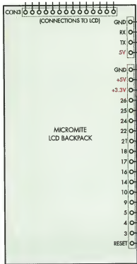
Fig.3: here's how to connect an e-Paper display to a Micromite. Only eight connections are required. Make sure you are not using the SPI bus for anything else, as this might conflict with the BASIC program.
