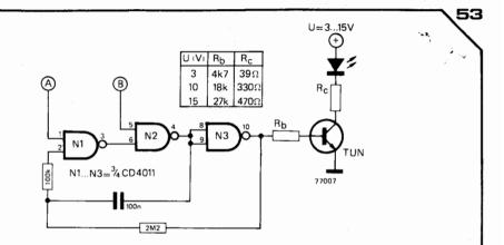
The condition of the LED is determined by the logic states of the two inputs A and B. If A is low and B is high then the LED will be lit continuously. If B is low then the LED will be extinguished, irrespective of the state of A. If A and B are both high then the
