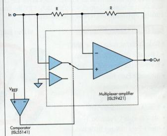
A multiplexer-amplifier IC combined with an external comparator offers a good alternative to a diode-bridge circuit for full-wave rectification. It saves board space while still allowing a relatively high operating frequency
