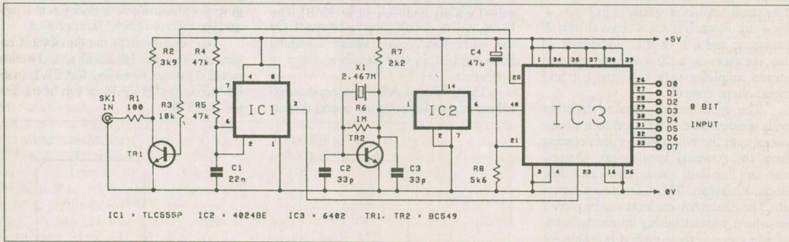
This circuit is based on the 6402 UART (IC3). A 4024 (IC2) and TR2 provide a clock circuit that gives a baud rate of 9600. A 555 oscillator is used to provide a continuous stream of pulses to the Transmitter Buffer Register Load input of the UART, and data is transmitted at something approaching the maximum rate possible for 9600 baud. The serial output at SK1 is similar to TTL level rather than
