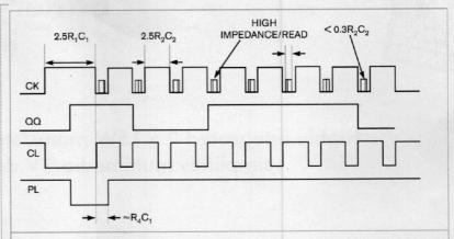
Figure 2 The high-impedance state must exist only for a time less than the R<sub>1</sub>C<sub>1</sub> time constant.
