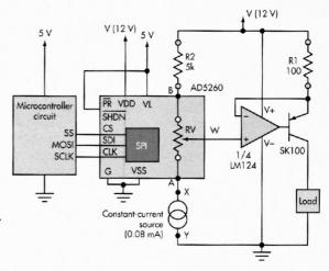
However, the digital potentiometer's wiper resistance is significant even when  $R_V$  is low, which introduces an error. To eliminate this error, the digital potentiometer is connected as a voltage divider, with the wiper resistance in series with the op amp's non-inverting input.
