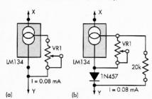
2. An adjustable current source and 2-k $\Omega$  potentiometer can be used in place of the fixed 0.08-mA constant-current source (a). The current source can also be adapted for use in an application with varying ambient temperature by adding a diode and 20-k $\Omega$  resistor.
