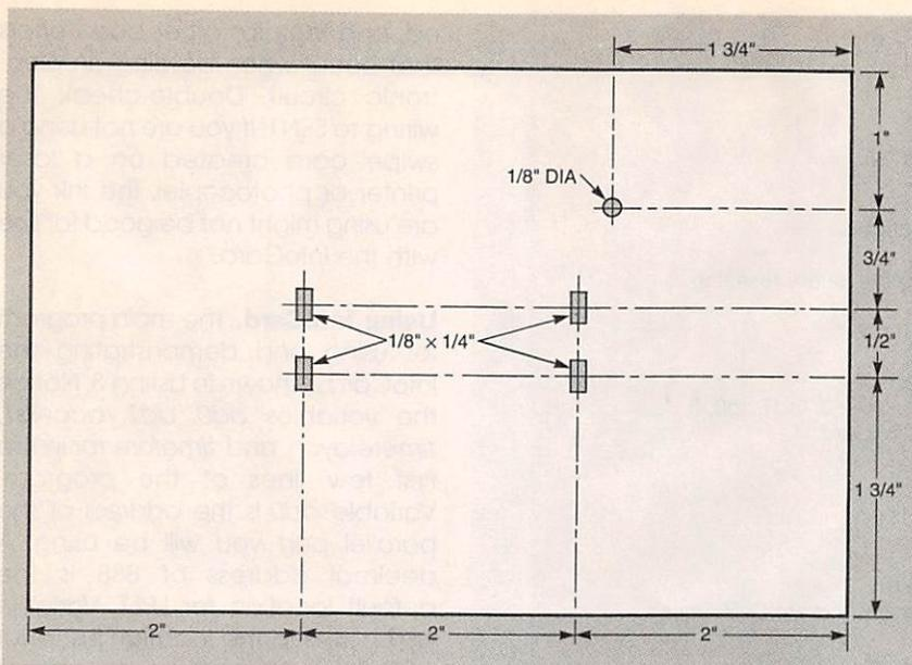
Fig. 5. The base plate has elongated slots so that the width of the card guide can be adjusted. The wires from the sensor pass through the hole in the upper corner. If you are going to use metal for the base plate, make that hole a bit larger and use a rubber grommet to protect the wires.
