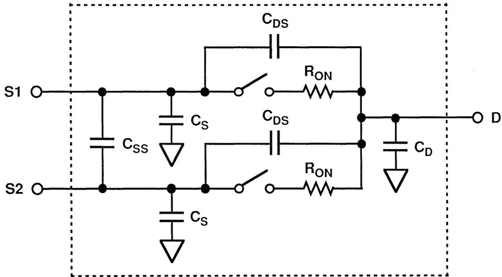
**Figure 7.34:** Channel-to-Channel Crosstalk Equivalent Circuit for Adjacent Switches
