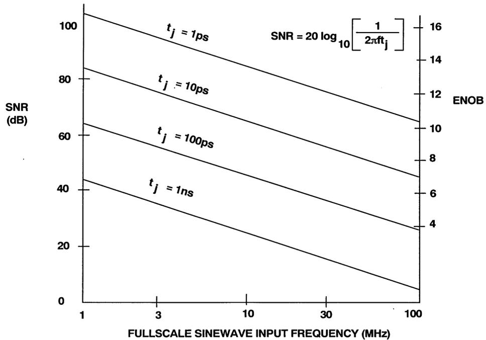
Figure 7.68: Effects of Sampling Clock Jitter on SNR
