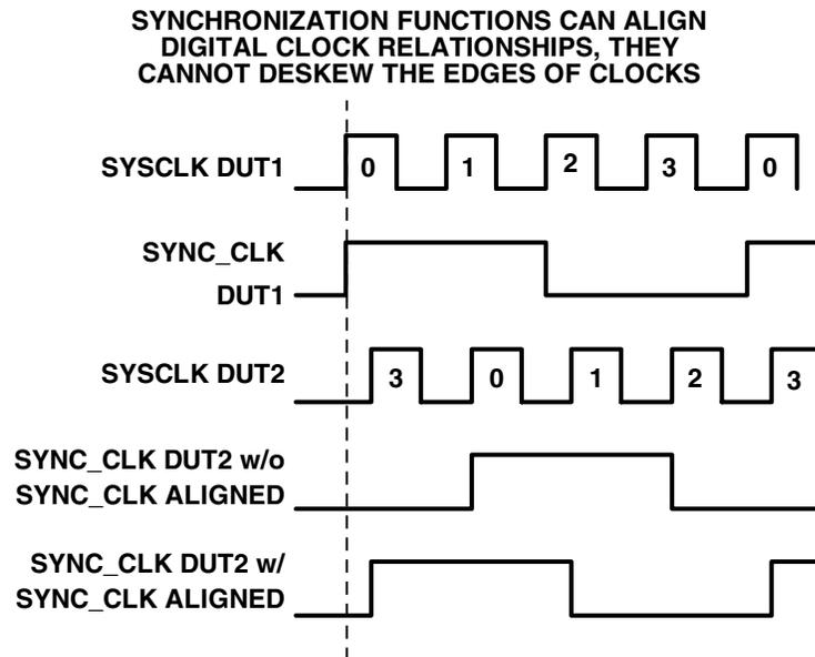
*Figure 7.78: Synchronization Functions: Capabilities and Limitations*
