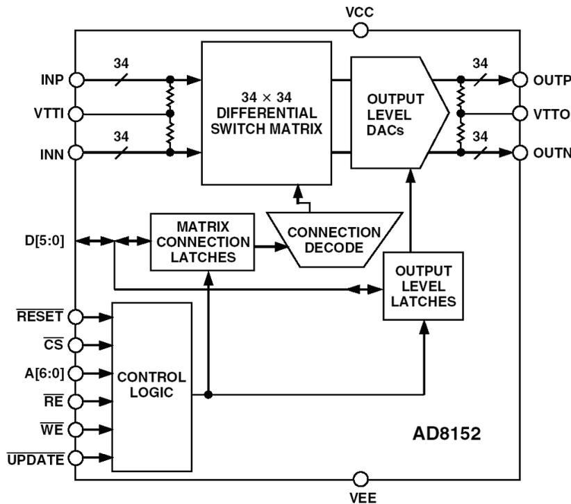
**Figure 7.53:** AD8152 3.2-Gbps Asynchronous Digital Crosspoint Switch
