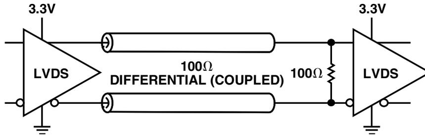
**Figure 7.89:** LVDS Output Termination
