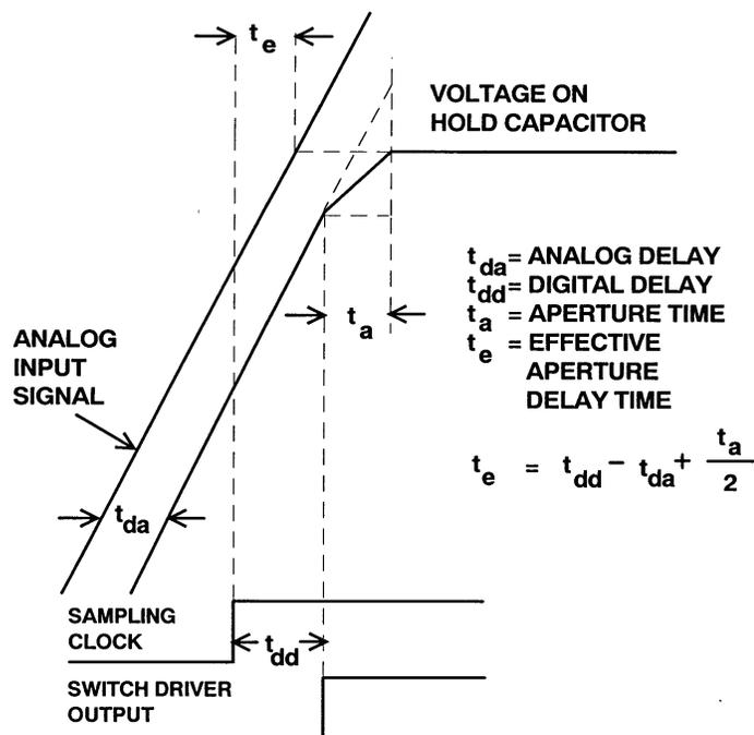
Figure 7.65: SHA Waveforms
