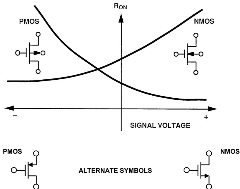
**Figure 7.18:** MOSFET Switch ON Resistance vs. Signal Voltage
