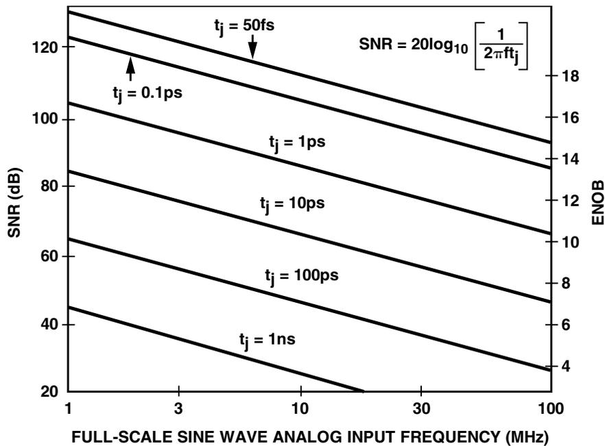
**Figure 7.74:** ENOB and SNR vs. Analog Input Frequency
