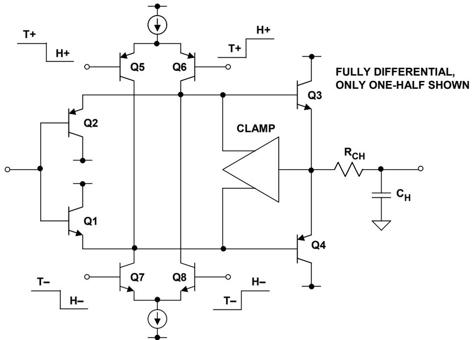
**Figure 7.73:** SHA Used in AD6645 14-Bit, 105 MSPS ADC
