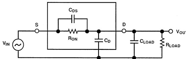
$$A(s) = \left[ \frac{R_{LOAD}}{R_{LOAD} + R_{ON}} \right] \left[ \frac{sR_{ON}C_{DS} + 1}{s \left( \frac{R_{LOAD}R_{ON}}{R_{LOAD} + R_{ON}} \right) (C_{LOAD} + C_D + C_{DS}) + 1} \right]$$
