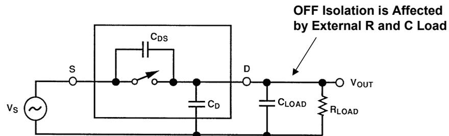
$$A(s) = \frac{s(R_{LOAD})(C_{DS})}{s(R_{LOAD})(C_{LOAD} + C_D + C_{DS}) + 1}$$
