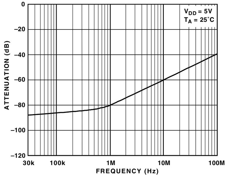
**Figure 7.35:** Crosstalk vs. Frequency for ADG708 8-Channel Multiplexer
