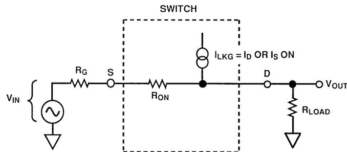
$$V_{OUT} = V_{IN} \left[ \frac{R_{LOAD}}{R_G + R_{ON} + R_{LOAD}} \right] + I_{LKG} \left[ \frac{R_{LOAD}(R_{ON} + R_G)}{R_G + R_{ON} + R_{LOAD}} \right]$$
