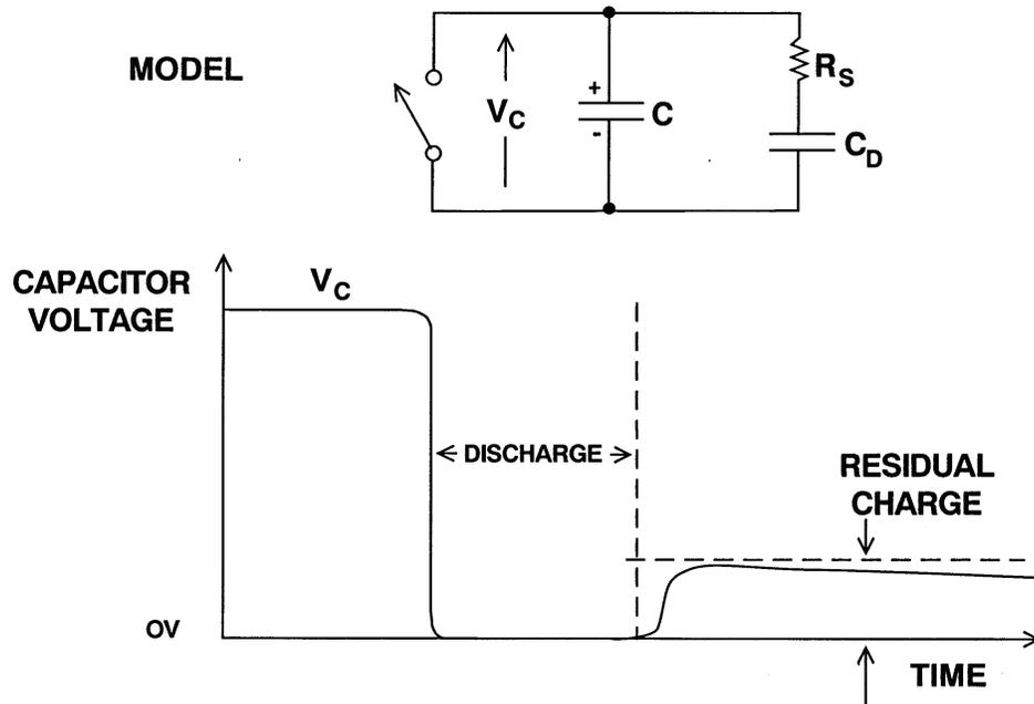
**Figure 7.70:** Dielectric Absorption
