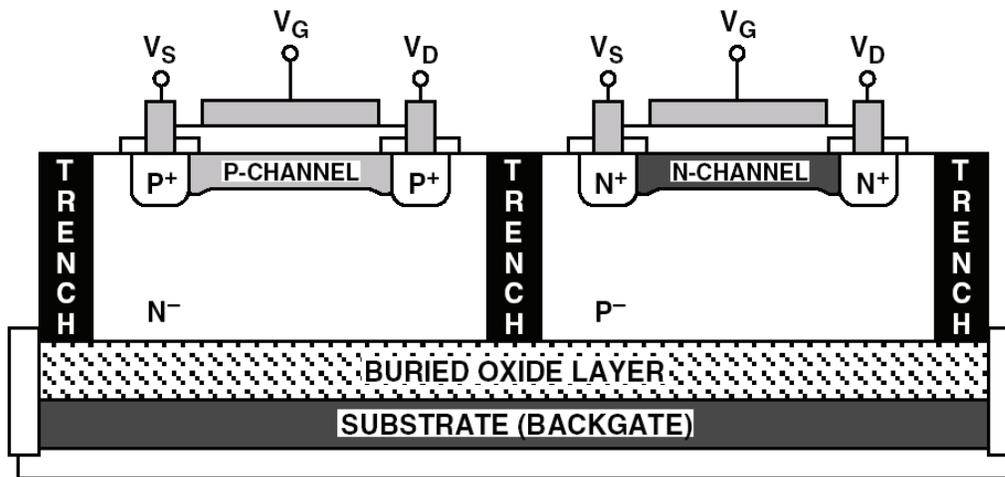
**Figure 7.59:** Trench-Isolation L<sup>2</sup>CMOS Structure
