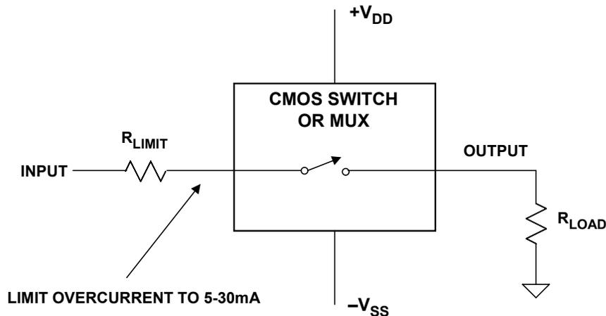
**Figure 7.57:** *Overcurrent Protection Using External Resistor*
