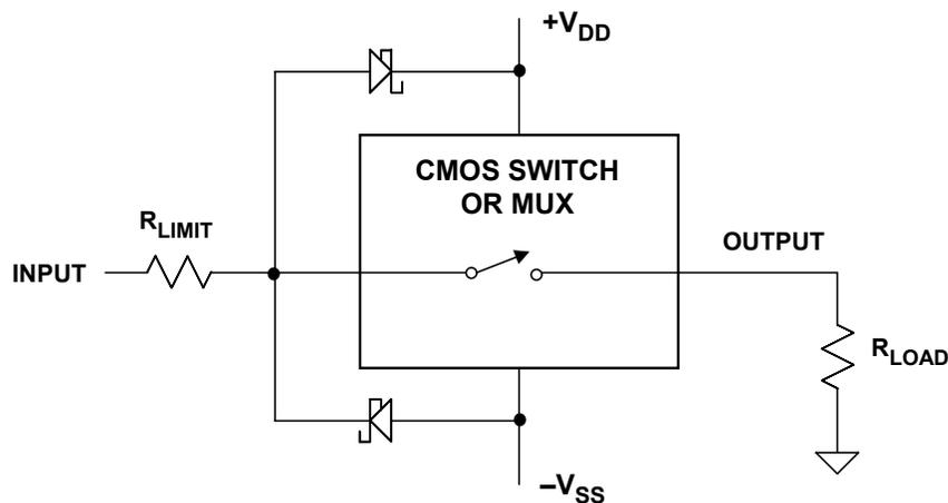
**Figure 7.58:** *Input Protection Using External Schottky Diodes*
