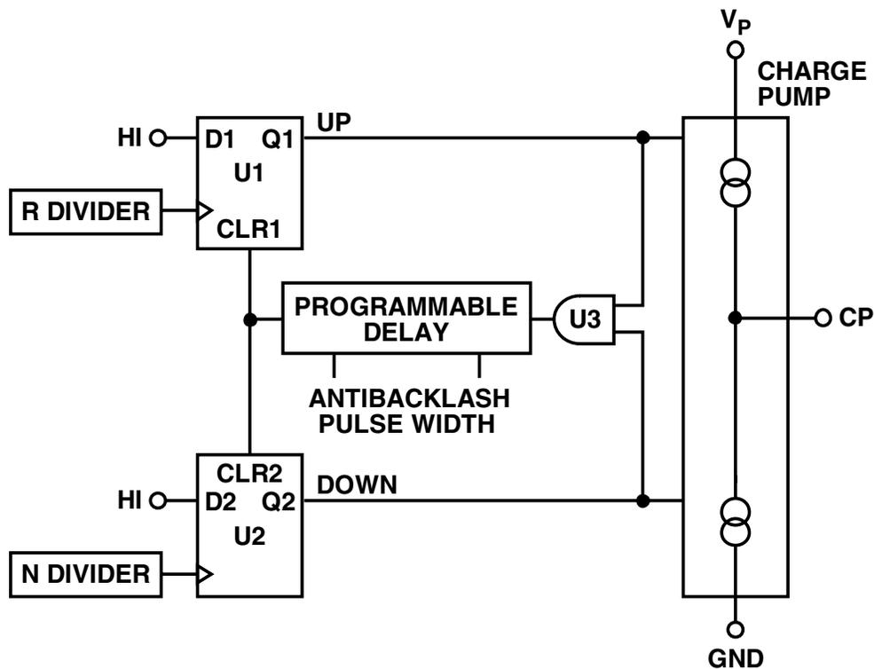
**Figure 7.82:** PFD Simplified Schematic and Timing (In Lock)
