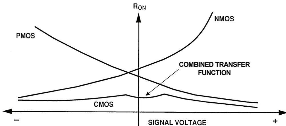
**Figure 7.20:** CMOS Switch ON Resistance vs. Signal Voltage
