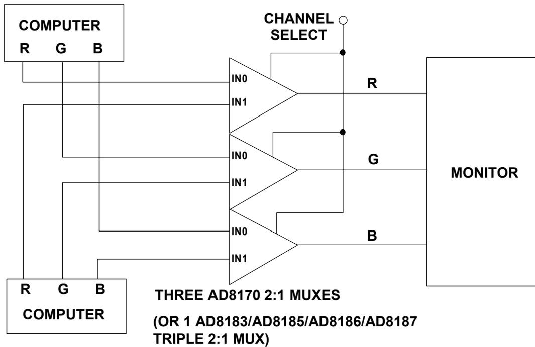
Figure 7.50: Dual Source RGB Multiplexer Using Three 2:1 Muxes
