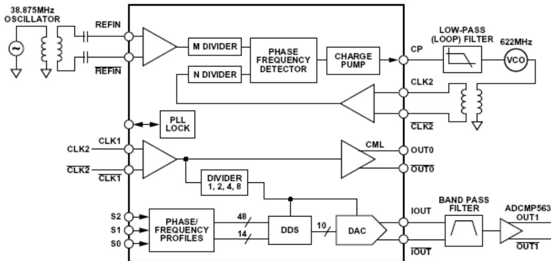
**Figure 7.76:** AD9540 Configured for Dual Clock Generation
