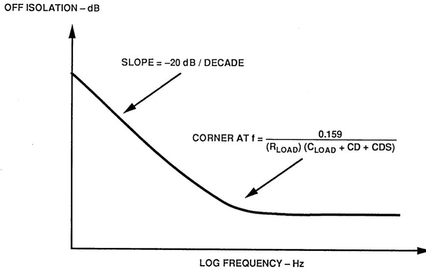
**Figure 7.28:** Off Isolation vs. Frequency
