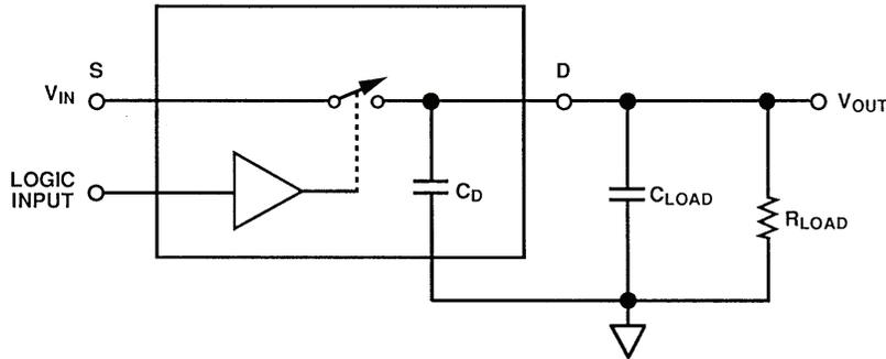
$$\text{OFF-TO-ON: } t_{\text{SETT}} = t_{\text{ON}} + \left( \frac{R_{\text{ON}} R_{\text{LOAD}}}{R_{\text{ON}} + R_{\text{LOAD}}} \right) (C_{\text{LOAD}} + C_{\text{D}}) \left( -\ln \frac{\% \text{ERROR}}{100} \right)$$
