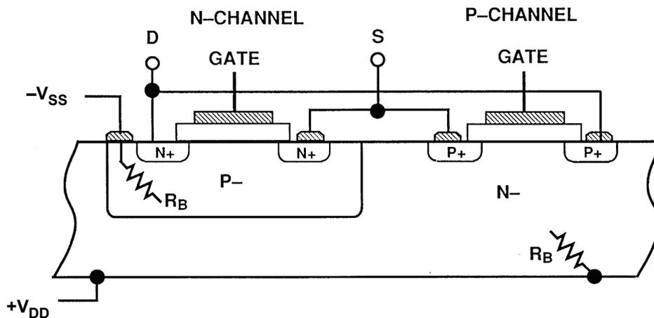
**Figure 7.54:** Cross-Section of a Junction-Isolation CMOS Switch
