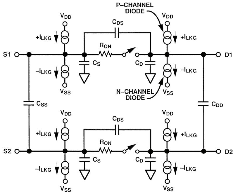
**Figure 7.22:** Equivalent Circuit of Two Adjacent CMOS Switches
