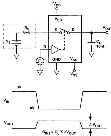
**Figure 7.31:** *Effects of Charge Injection on Output*
