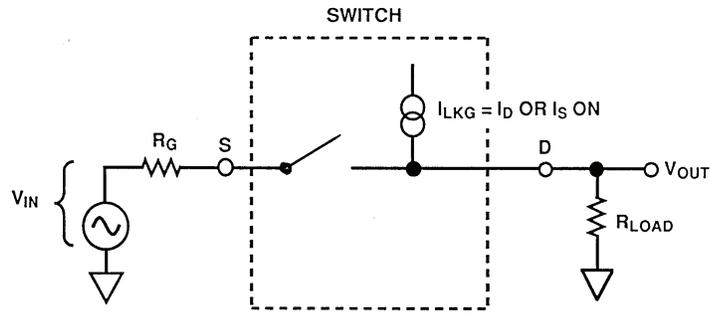
Leakage current creates error voltage at  $V_{OUT}$  equal to:
