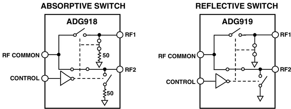
Figure 7.46: 1-GHz CMOS 1.65-V to 2.75-V 2:1 Mux/SPDT Switches
