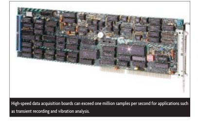
A/D converter might require 2.5 ms, making the maximum sampling rate a fairly slow 400 Hz.
