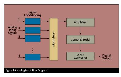
fused with its absolute accuracy! Amplification of the signal, or input gain, can be used to increase the apparent sensitivity if the signal's expected maximum range is less than the input range of the A/D converter. Because higher resolution A/D converters cost more, it is especially important to not buy more resolution than you need—if you have 1% accurate (1 in 100) temperature transducers, a 16-bit (1 in 65,536) A/D converter is probably more resolution than you need.
