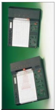
Flatbed recorders offer a portable, flexible alternative to permanently mounted units.
