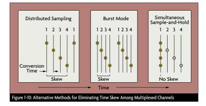
does reduce the frequency with which data points are acquired, and that the Nyquist sample-rate criterion still must be observed. During a typical data acquisition process, individual channels are read in turn sequentially. This is called standard, or distributed, sampling. A reading of all channels is called a scan. Because each channel is acquired and converted at a slightly different time, however, a skew in sample time is created between data points (Figure 1-10).
