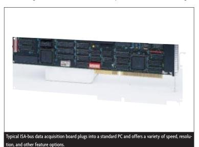
In addition to comparing basic specs, examine how the product is designed and built. Accuracy is often dependent upon the amount of noise picked up by the system. Modern data acquisition products minimize this problem in several ways:
