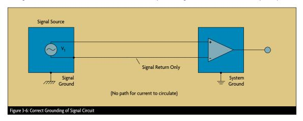
a stable reference for making voltage measurements. Ground wires also safeguard against unwanted common-mode signals and prevent accidental contact with dangerous voltages. Return lines carry power or signal currents (Figure 3-4). A ground loop is a potentially dangerous loop formed when two or more points in an electrical system are grounded to different potentials.
