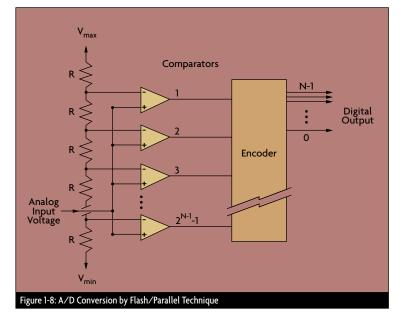
for. This design uses multiple comparators in parallel to process samples at more than 100 MHz with 8 to 12-bit resolution. Conversion is accomplished by a string of comparators with appropriate references operating in parallel (Figure 1-8).
