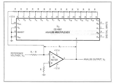
**D-a converter.** Analog multiplexer  $U_2$  places resistors in the feedback path of amplifier  $U_1$  to control the latter's gain and thereby produce an output proportional to the digital input. The analog output  $V_0 = -NV_R$ , where N is the decimal equivalent of the digital input and  $V_B$  is the reference voltage.
