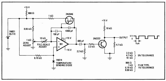
**Temperature-to-frequency converter.** Frequency of relaxation oscillator varies with temperature-dependent voltage across 1N914 diode. Over 0°C-to-100°C temperature range, frequency changes linearly from 0 to 1,000 Hz. Therefore frequency meter at output can show temperature directly. Accuracy is ±0.3°C. Excellent performance and low cost (less than \$5 for parts) make this circuit outstanding.
