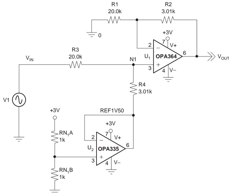
**Figure 3. Circuit 2: Single-Supply/Single-Part**
