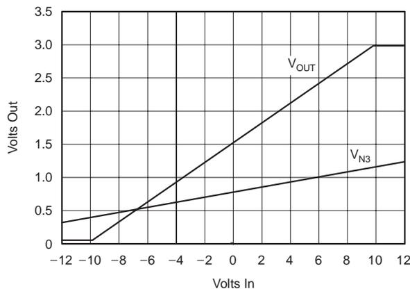
**Figure 10. DC Sweep of Circuit 5**
