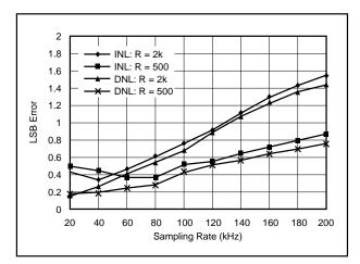
FIGURE 2. If the Resistors  $(R_1 \text{ and } R_2)$  are High Enough They can Cause Errors at Higher Sampling Frequencies.
