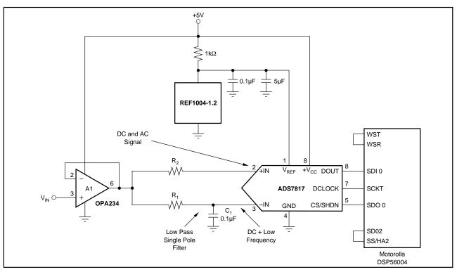
FIGURE 1. The ADS7817 in Conjunction with an R || C Network is Used to Reject DC Pedestal Voltages in a Single Supply Environment and Digitize the ac Portion of the Analog Signal. The REF1004-1.2 is a 1.2 voltage reference for the A/D converter, providing a full-scale range of 2.4Vp-p and theoretical LSB size of 0.6mV.
