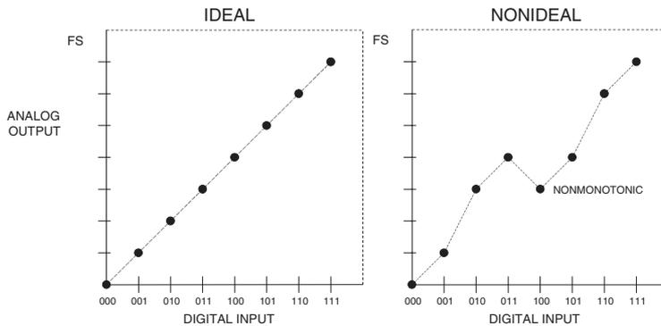
Figure 3-6: DAC transfer functions
