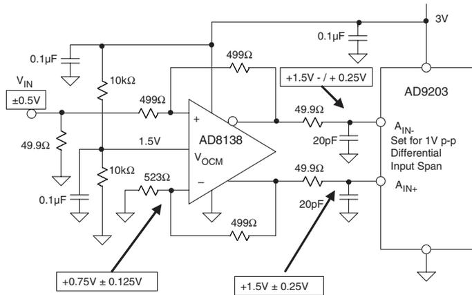
Figure 3-44: AD8138 driving AD9203 10-bit, 40 MSPS ADC
