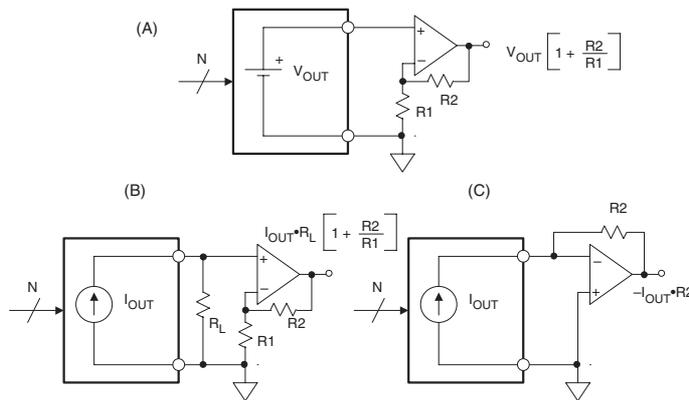
Figure 3-51: Buffering DAC outputs with op amps
