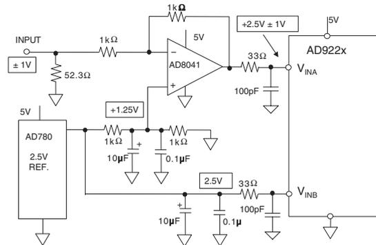
**Figure 3-38: Dc-coupled single-ended, single-supply ADC driver/level shifter using external reference**
