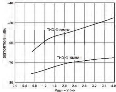
On the other hand, Figure 3-25 shows distortion as a function of output signal level for a frequencies of 5 MHz and 20 MHz.
