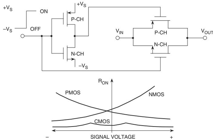
Figure 3-28: Basic CMOS analog switch
