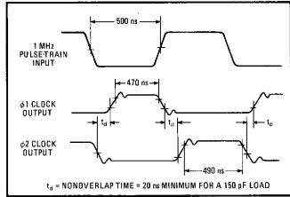
**2. No overlap.** With a 1-MHz, 50%-duty-cycle input signal, the  $\phi_1$  and  $\phi_2$  outputs have durations of 470 ns and 490 ns, respectively. The nonoverlap, which is dependent upon the propagation delay of the gates, is a function of load capacitance and varies from about 10 ns with a 15-pF load to 20 ns with a 150-pF load.
