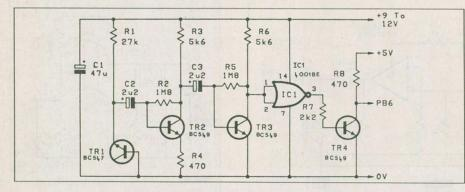
This simple method of producing a random clock signal uses a reverse-biased emitter-base junction that emits noise spikes in much the same way as a zener diode. TR2 and TR3 provide voltage gain for the very low-amplitude spikes (these can be any general-purpose NPN). The 4001BE NOR gate cleans up the signal to CMOS level; if you need a CMOS level, take the signal from pin 3 of the 4001. If you need TTL levels, take the output from the collector of TR4, which can also be any general purpose NPN.
