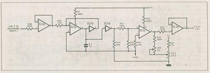
Useful for synthesizers or test gear, this linear-to-logarithmic converter uses the LM 13600 transconductance amplifier (IC1) and any dual low-noise op amp. To maintain the same equivalent currents on both control nodes of IC1a and 1c, which assists temperature stability, the gain can be varied with trimmer VR5 to change the load factor at the output of IC1c. The overall voltage range can be shifted up or down by adjusting trimmer VR3.
