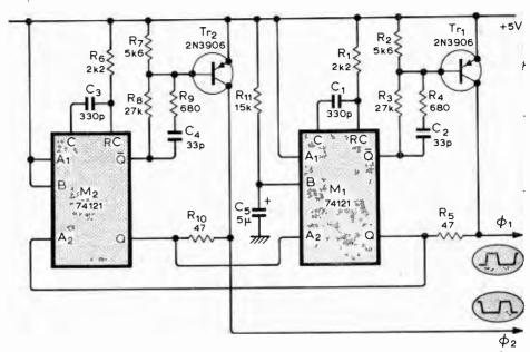
will be no spare A inputs to 5V, but the spare clear inputs must be tied to the supply rail. Also,  $R_1$  and  $R_6$  should be increased to  $3k9\Omega$ . The circuit will drive loads of 150pF and keep within Motor-
