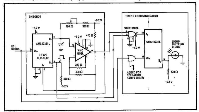
Hot shot. Spotting timing errors in a fast one-shot multivibrator is simplified with the addition of an error indicator circuit such as the one shown in the shaded area. If the clock rate is too high or the output pulse width is too small, the LED will indicate it
