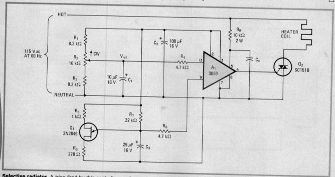
**Selective radiator.** A triac fired by this controller applies power to and removes power from heater coil of hot plate during zero crossings of the 115-V ac power line, thus eliminating unwanted electrical hash and noise formerly caused by mechanical-type thermal switches. User sets temperature with duty-cycle control  $R_2$ , which turns on  $A_1$  and triac when  $V_{ref}$  is less than the instantaneous ramp output of oscillator  $Q_1$ .
