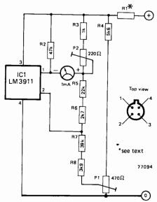
supply voltage is not critical provided the value of R1 is chosen so that about 3 mA flows through it. The value of R1 is given by
