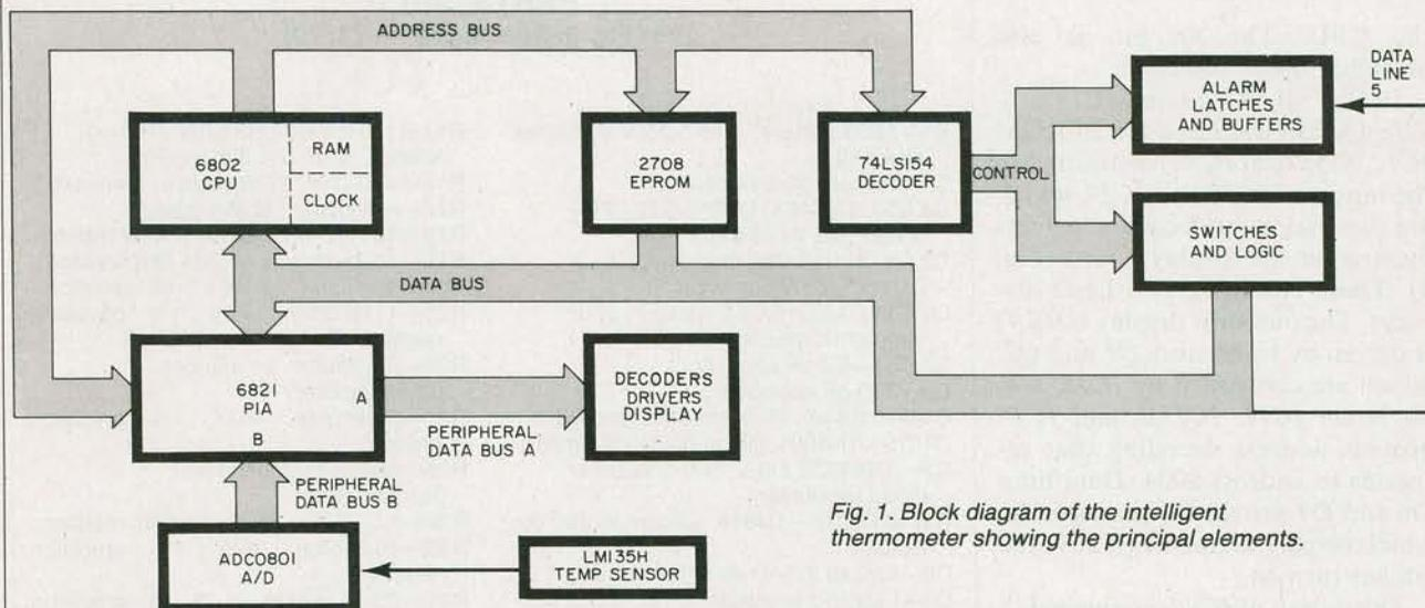
Fig. 1. Block diagram of the intelligent thermometer showing the principal elements.
