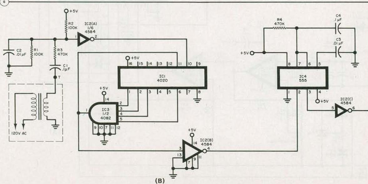
Fig. 3B. EPROM and logic circuits.
