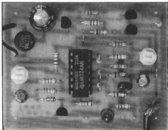
***This solid-state thermostat can replace those old mechanical units—at a cost of less than twenty dollars!***
