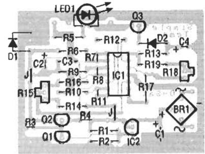
FIG. 2—PARTS-PLACEMENT DIAGRAM. Any method of construction can be used, but it's best to use a PC board. You can make one from the foil pattern we've provided or buy one from the source mentioned in the Parts List.
