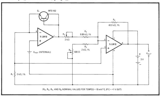
**Hot number.** Micropower op amp and semiconductor made specifically for temperature-sensing applications reduce complexity and calibration procedure of thermometers that use  $V_{be}$  of transistors to detect temperature changes. Accuracy of device, no worse than  $\pm 2^{\circ}$ C over the range of  $-40^{\circ}$ C to  $+150^{\circ}$ C, and its simplicity enable it to compete with much more expensive units.
