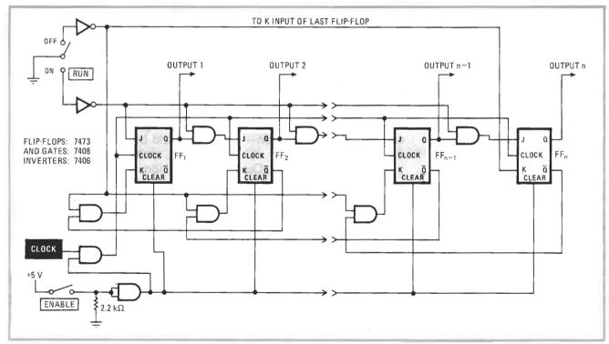
**First on, last off.** With ENABLE switch on, turning RUN switch on starts the latching sequence: with each clock pulse Q output of each flip-flop goes high in ascending order, until all are high. Turning RUN switch off unlatches outputs in descending order. The circuit was designed to permit switching of antenna couplers only after removing power from radio transmitter, and RUN function was performed by keying.
