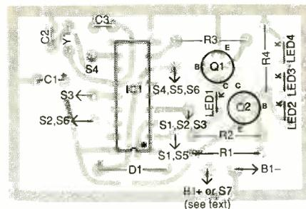
Fig. 9. Wiring guide for transmitter pc board.
