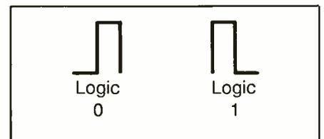
Fig. 3. Position of amplitude modulation for each bit of the word determines if bit is a 1 or a 0.
