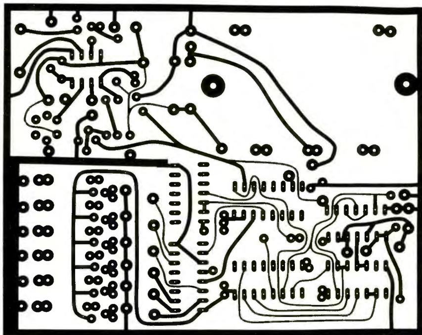
Fig. 8. Actual-size etching-and-drilling guide for receiver/decoder pc board.
