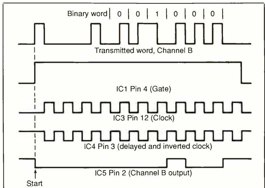
Fig. 6. Decoder circuit timing diagram.
