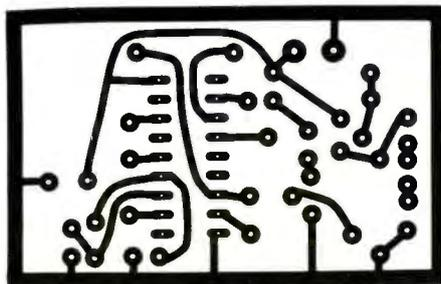
Fig. 7. Actual-size etching-and-drilling guide for transmitter pc board.
