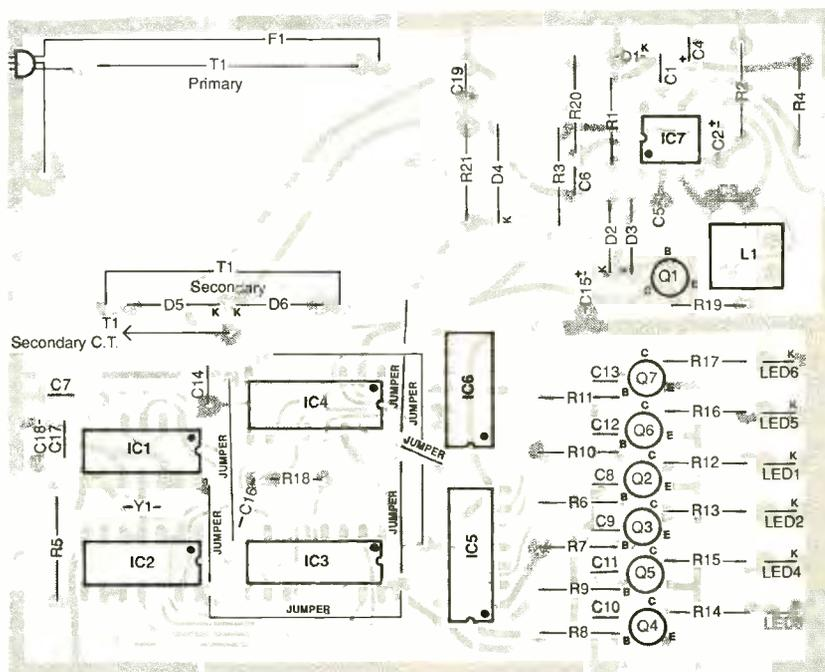
Fig. 10. Wiring guide for receiver/decoder pc board.
