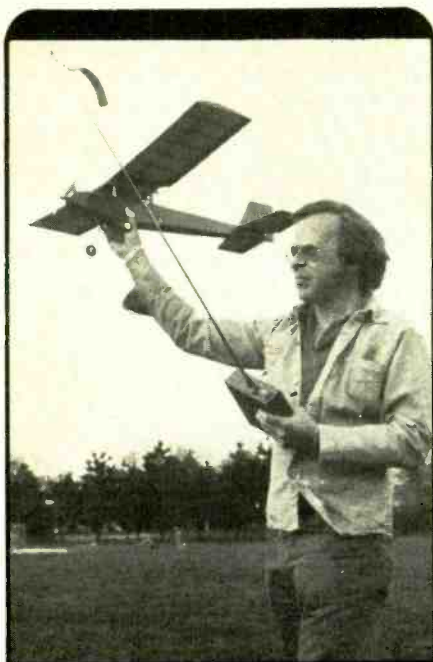
Les Shine launches his Cox Q-Tee airplane with one hand while maintaining radio control with the other. The plane is highly maneuverable, permitting its use in relatively small areas.
