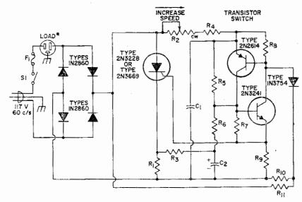
\* Maximum load is 2 amperes when 2N3228 SCR is used or 12.5 amperes when 2N3669 SCR is used.
