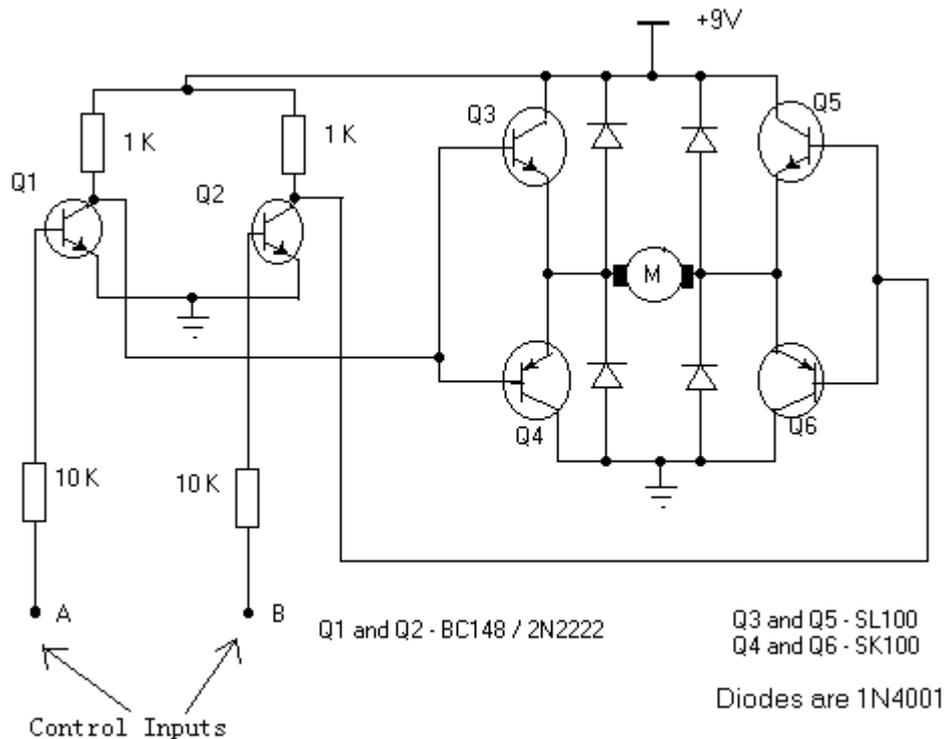
CAUTION: The max motor current rating not to exceed max. SL/SK100 rating (1A with heat sink)
