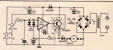
The disadvantage of most simple speed controllers for model trains or cars is that they simply supply the motor with a fixed voltage. Consequently the speed does not remain constant, since the model slows down when climbing gradients and speeds up when going downhill. With model trains the setting of the control knob to maintain a particular speed also varies with the load that the engine is pulling.
