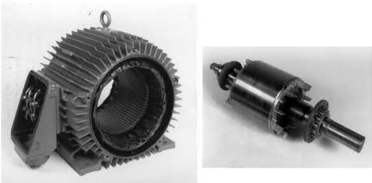
**FIG. 5.12** Cage rotor for induction motor. The rotor conductor bars and end rings are cast in aluminium, and the blades attached to the end rings serve as a fan for circulating internal air. An external fan will be mounted on the nondrive end to cool the finned stator casing (as shown in Fig. 8.4).
