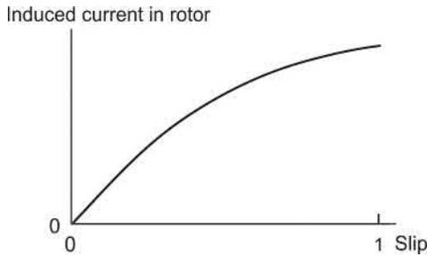
**FIG. 5.19** Magnitude of current induced in rotor over the full (motoring) range of slip.
