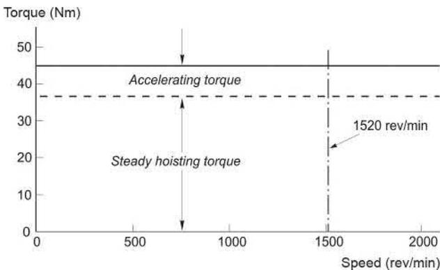
FIG. 11.8 Torque requirements for motor in hoist application (Fig. 11.7).
