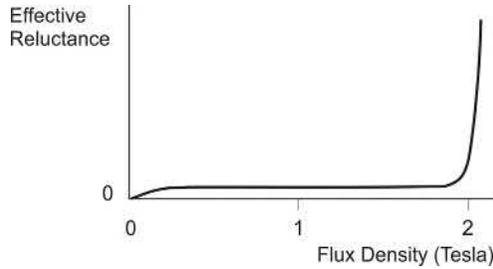
**FIG. 1.10** Sketch showing how the effective reluctance of iron increases rapidly as the flux density approaches saturation.
