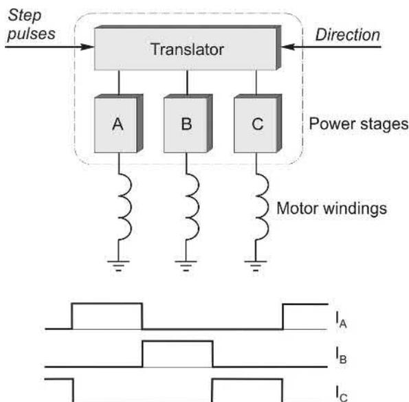
**FIG. 10.12** General arrangement of drive system for 3-phase motor, and winding currents corresponding to an 'ideal' drive.
