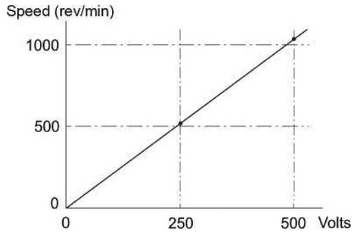
**FIG. 3.7** No-load speed of d.c. motor as a function of armature voltage.
