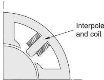
**FIG. 3.5** Sketch showing location of interpole and interpole winding. (The main field windings have been omitted for the sake of clarity.)
