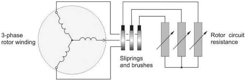
**FIG. 5.13** Schematic diagram of wound rotor for induction motor, showing sliprings and brushes to provide connection to the external (stationary) three-phase resistance.
