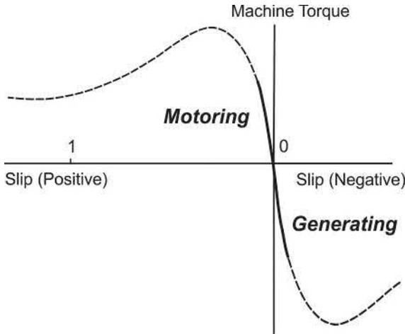
FIG. 5.22 Typical torque-speed characteristic showing stable motoring and generating regions.
