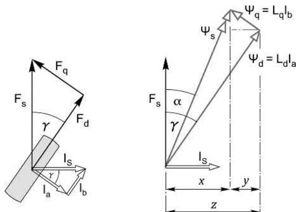
FIG. 9.10 Reluctance motor—axis m.m.f.'s and flux linkages.
