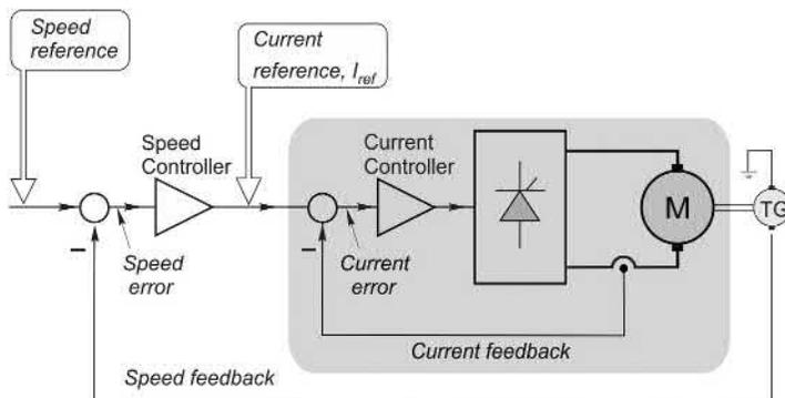
**FIG. 4.12** Schematic diagram of analogue controlled-speed drive with current and speed feedback control loops.
