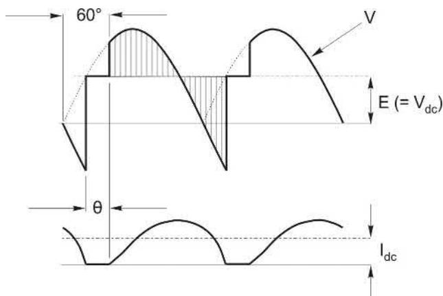
**FIG. 4.4** Armature voltage and current waveforms for discontinuous-current operation of a d.c. motor supplied from a single-phase fully-controlled thyristor converter, with firing angle of 60 degrees.
