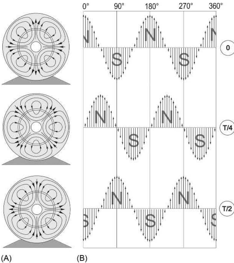
**FIG. 5.1** (A) Flux pattern in a four-pole induction motor at three successive instants of time, each one-quarter of a cycle apart; (B) radial flux density distribution in the air-gap at the three instants shown in Fig. 5.1A.
