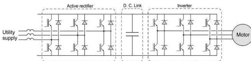
FIG. 2.26 A.C. motor drive with active front-end rectifier.
