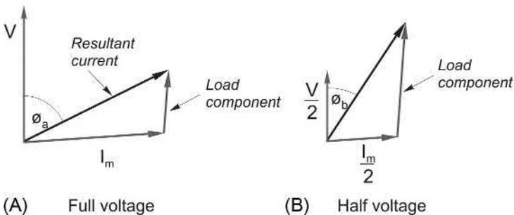
FIG. 6.23 Phasor diagram showing improvement of power-factor by reduction of stator voltage.
