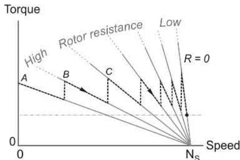
**FIG. 6.14** Torque-speed curves for a wound-rotor (slipping) motor showing how the external rotor-circuit resistance ( $R$ ) can be varied in steps to provide an approximately constant torque during acceleration.
