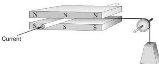
FIG. 1.14 Primitive linear d.c. motor.
