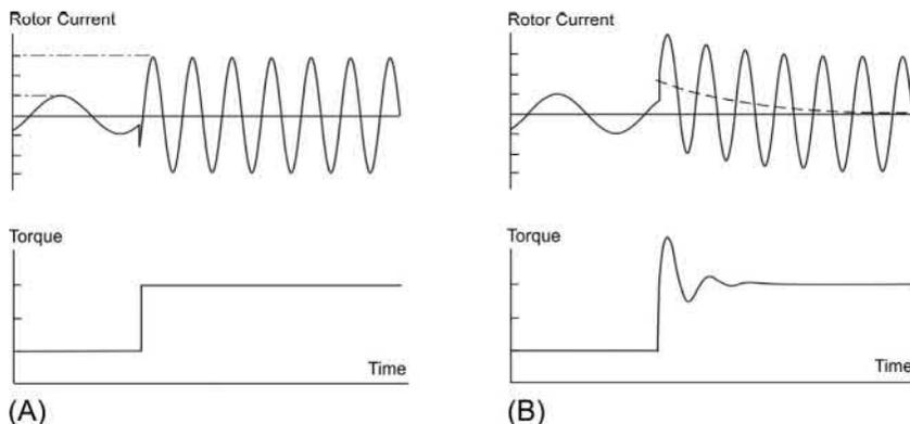
**FIG. 8.12** Step changes in rotor current. (A) Transient-free transition with correct changes to magnitude, frequency and instantaneous position of stator m.m.f. wave (i.e. vector control). (B) Same changes to magnitude and frequency, but not phase.
