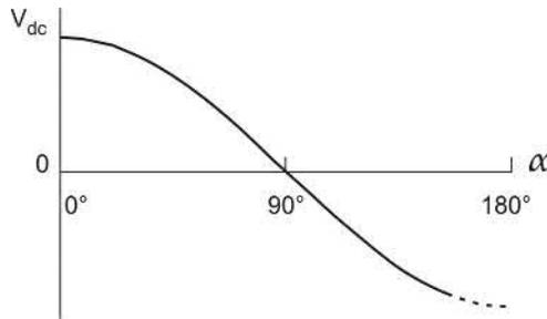
**FIG. 4.7** Average d.c. output voltage from a fully-controlled thyristor converter as a function of the firing angle delay  $\alpha$ .
