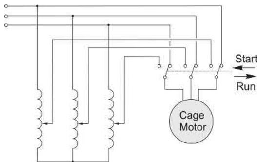
FIG. 6.3 Autotransformer starter for cage induction motor.
