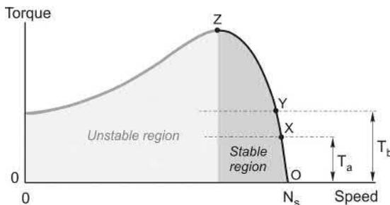
FIG. 6.10 Torque-speed curve illustrating stable operating region (OXYZ).
