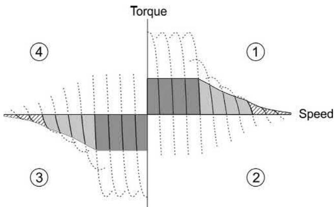
FIG. 7.7 Operating regions in all four quadrants of the torque-speed plane.
