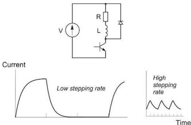
FIG. 10.15 Basic constant-voltage drive circuit and typical current waveforms.
