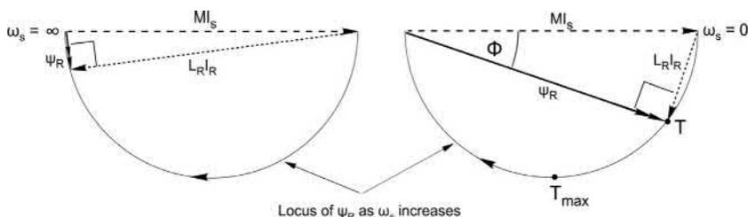
FIG. 8.7 Locus of rotor flux linkage space phasor as slip frequency varies.
