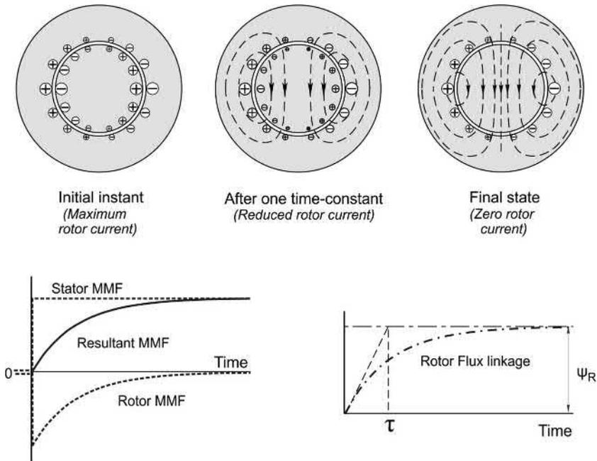
FIG. 8.11 Diagrams illustrating the build-up of rotor flux when a step of stator m.m.f. occurs.
