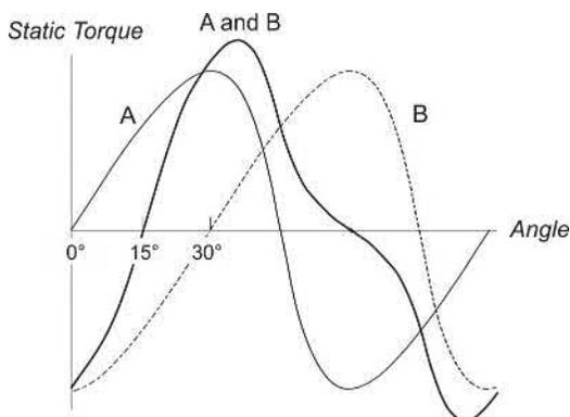
FIG. 10.11 Static torque curve (solid line) corresponding to two-phase-on excitation.
