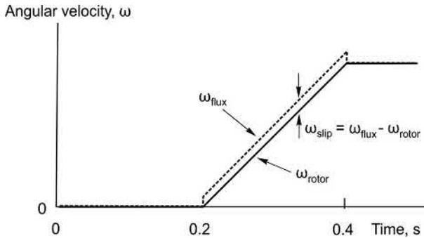
FIG. 8.23 Angular velocity during acceleration.
