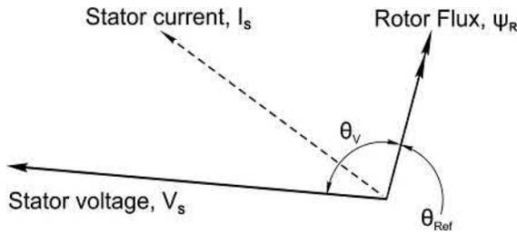
FIG. 8.20 Time phasor diagram showing stator voltage and current under steady-state conditions.
