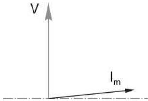
**FIG. 5.10** Phasor diagram for the induction motor under no-load conditions, showing magnetising current  $I_m$ .
