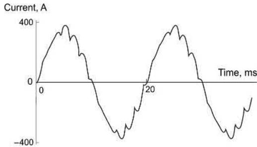
FIG. 7.18 Utility supply current waveform for 150kW drive with 12-pulse rectifier.
