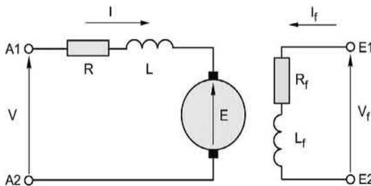
FIG. 3.6 Equivalent circuit of a d.c. motor.
