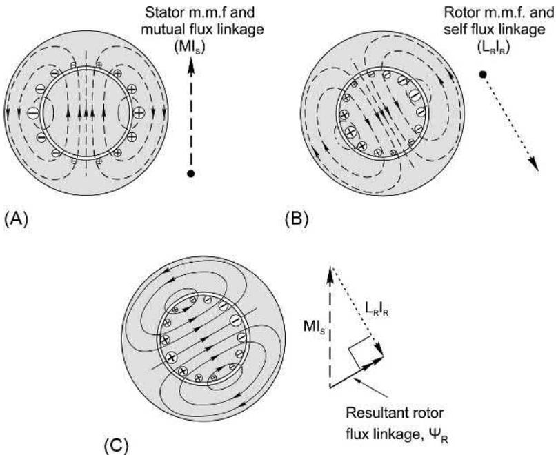
FIG. 8.6 Space phasors of m.m.f. and flux linkage under locked-rotor conditions.
