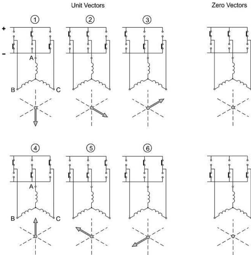
FIG. 8.13 Voltage phasors for all acceptable combinations of switching for a 3-phase inverter.
