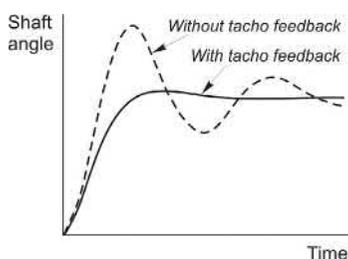
**FIG. 4.17** Typical step responses for a closed-loop position control system, showing the improved damping obtained by the addition of tachometer feedback.
