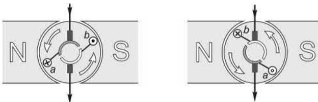
**FIG. 3.4** Simplified diagram of single-coil motor to illustrate the current-reversing function of the commutator.
