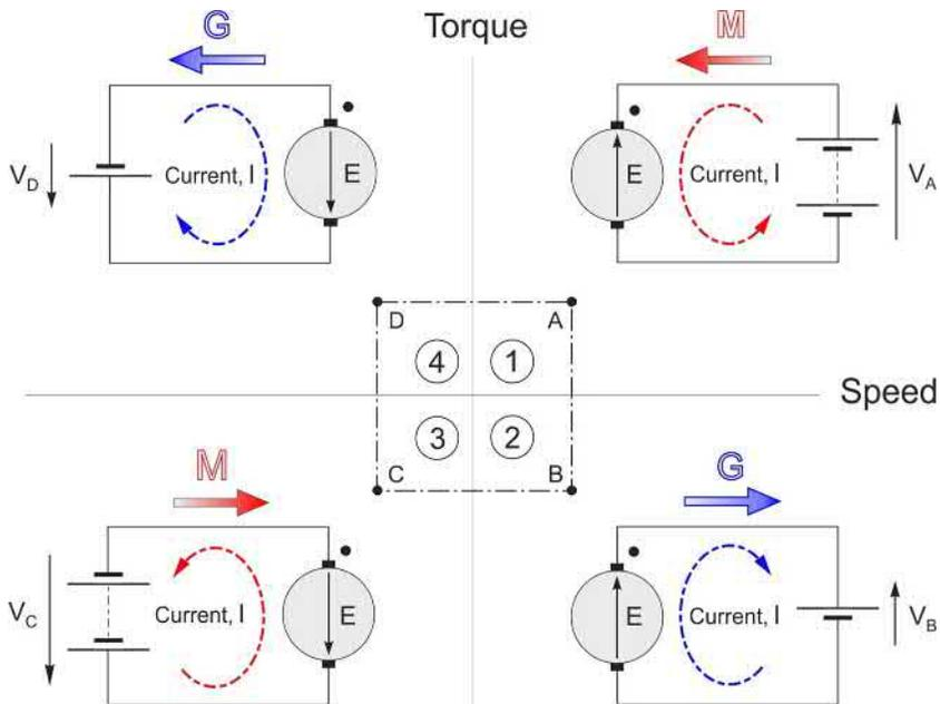
FIG. 3.12 Operation of d.c. motor in the four quadrants of the torque-speed plane.
