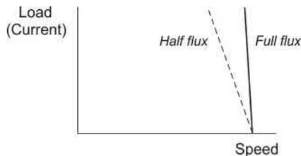
**FIG. 1.20** Influence of flux on the drop in steady running speed when load is applied.
