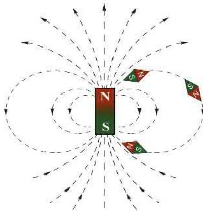
FIG. 1.2 Magnetic flux lines produced by a permanent magnet.
