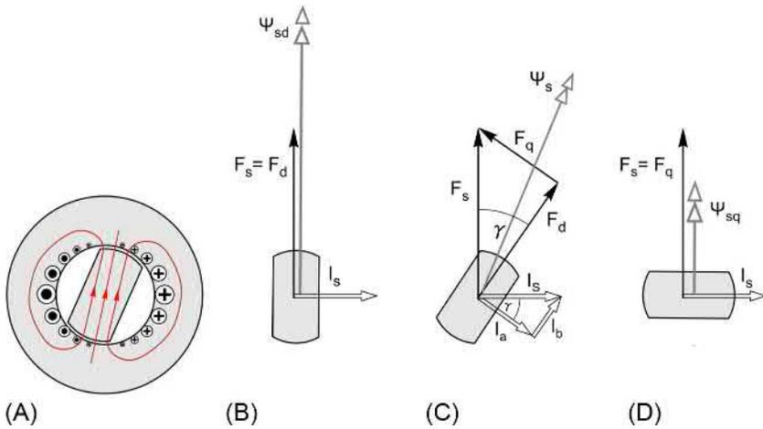
FIG. 9.9 Space phasors for a reluctance motor.
