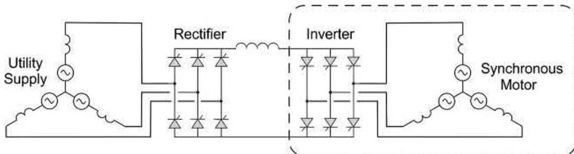
FIG. 9.24 Converter-fed large excited-rotor synchronous machine drive.
