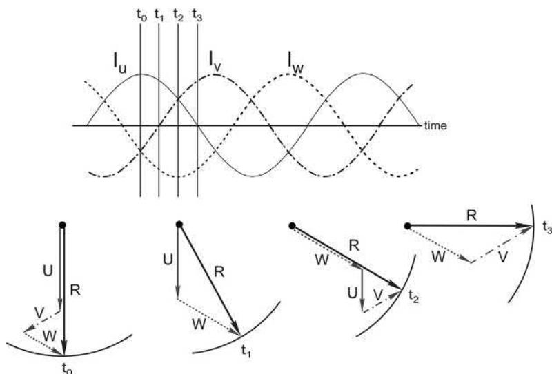
**FIG. 8.2** Resultant m.m.f. space phasor for balanced 3-phase operation at four discrete times, each separated by one-twelfth of a cycle (i.e.  $30^\circ$ ).
