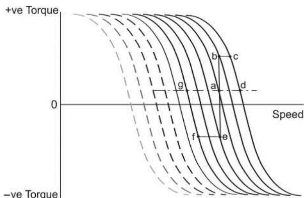
FIG. 7.6 Acceleration and deceleration trajectories in the torque-speed plane.
