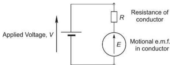
FIG. 1.16 Equivalent circuit of primitive d.c. motor.
