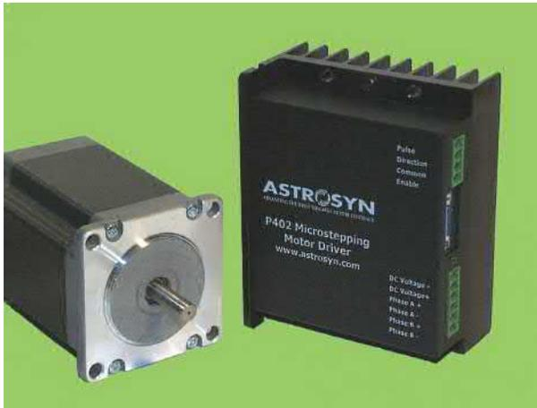
**FIG. 10.19** Bipolar drive with integral heatsink providing a range of step divisions up to 25,600steps/rev. It allows drive current to be set from 0.25 A to 2.0 A with supply voltage from 14 V to 40 V. (Courtesy of Astrosyn International Technology Ltd.)
