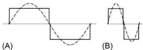
FIG. 2.15 Single-phase inverter output voltage waveforms—resistive load.
