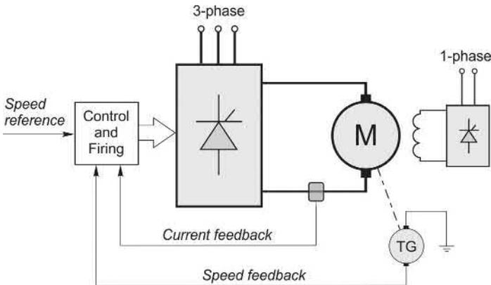
FIG. 4.1 Schematic diagram of speed-controlled d.c. motor drive.
