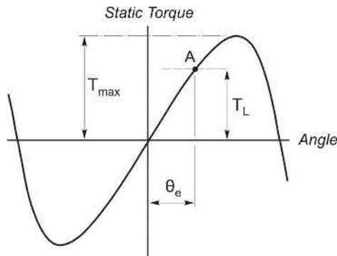
FIG. 10.10 Static torque–angle curve showing step position error ( $\theta_e$ ) resulting from load torque  $T_L$ .
