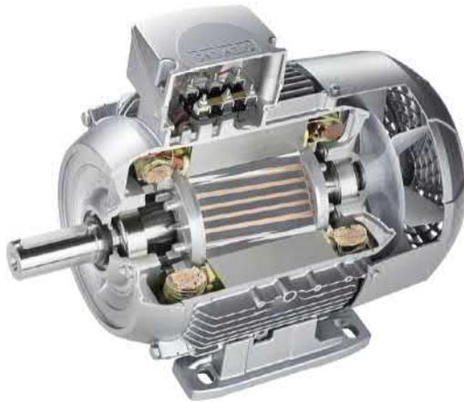
**FIG. 6.9** Cutaway view of cage induction motor showing skewed rotor bars. The bars are of cast aluminium, and the paddles attached to the end rings serve as a fan for circulating internal air. The external fan mounted on the non-drive end cools the finned stator casing. (Courtesy of Siemens.)
