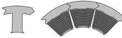
FIG. 9.38 Segmented stator.
