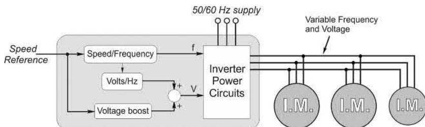
FIG. 7.11 Simple V/f induction motor control strategy applied to a multi-motor system.
