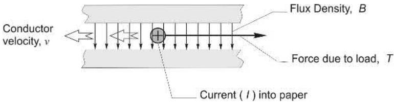
FIG. 1.15 Diagrammatic sketch of primitive linear d.c. motor.
