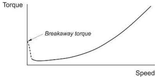
FIG. 11.9 Torque-speed characteristics for fan-type load.
