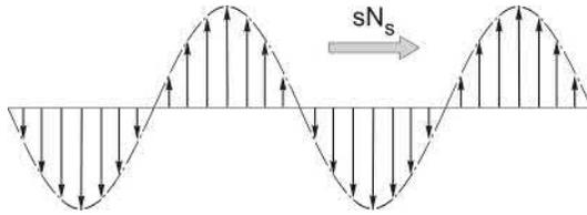
FIG. 5.15 Pattern of induced e.m.f.'s in rotor conductors. The rotor 'voltage wave' moves at a speed of  $sN_s$  with respect to the rotor surface.
