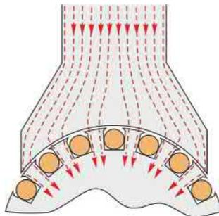
FIG. 1.13 Influence on flux paths when the rotor is slotted to accommodate conductors.
