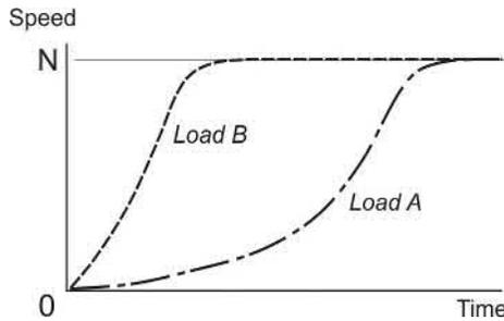
**FIG. 6.6** Speed-time curves during run-up, for motor and loads shown in Fig. 6.5.
