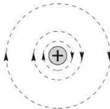
FIG. 1.5 Magnetic flux lines produced by a straight, current-carrying wire.
