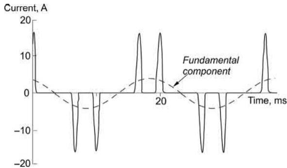
FIG. 7.13 Typical current from utility supply for a 1.5kW 3-phase drive.
