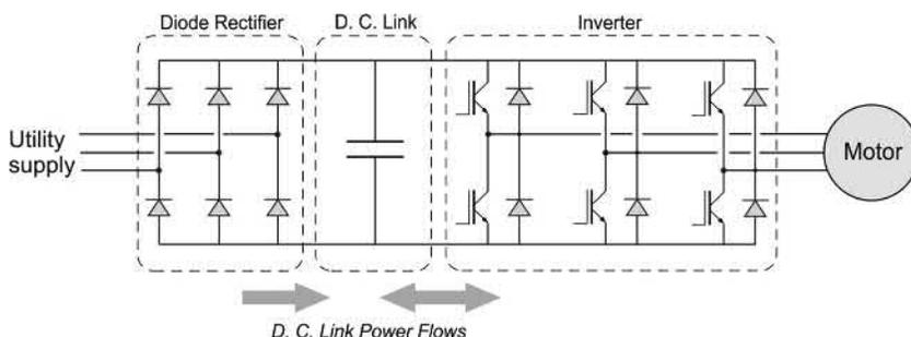
**FIG. 7.8** Pulse-width modulated (PWM) voltage source inverter (VSI).
