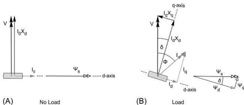
FIG. 9.17 Time phasor diagrams for the reluctance motor.
