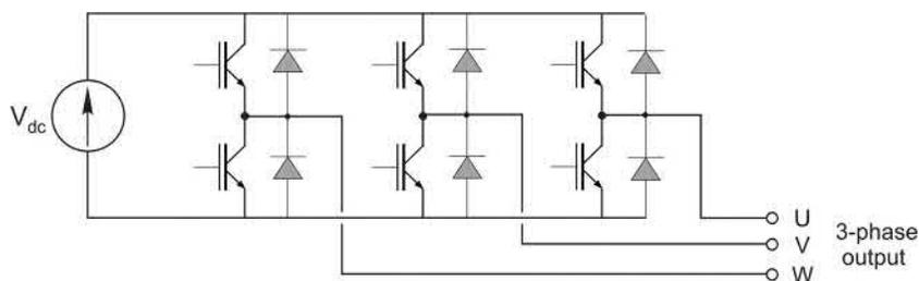
**FIG. 9.28** Three-phase inverter power circuit.
