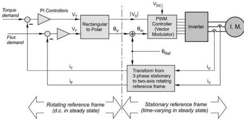
FIG. 8.16 Simplified block diagram of a typical field-oriented torque control system.
