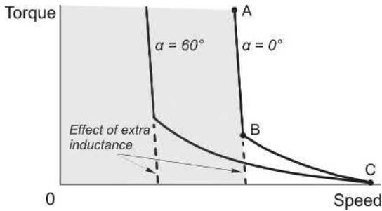
**FIG. 4.5** Torque-speed curves illustrating the undesirable 'droopy' characteristic associated with discontinuous current. The improved characteristic (shown dotted) corresponds to operation with continuous current.
