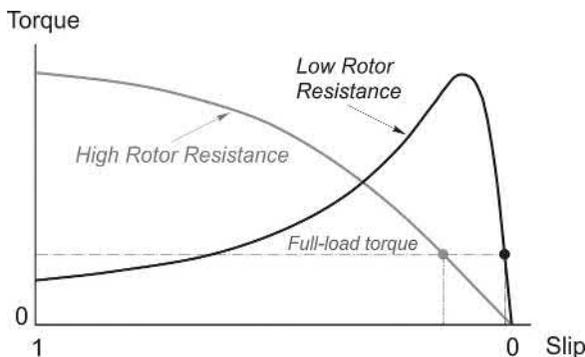
FIG. 6.11 Influence of rotor resistance on torque-speed curve of cage motor. The full-load running speeds are indicated by the vertical dotted lines.
