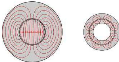
**FIG. 9.37** Comparison of 2-pole and 8-pole stator cores.
