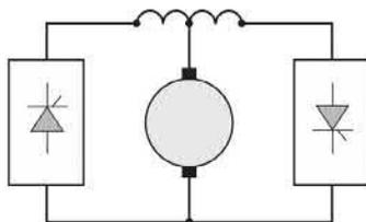
FIG. 4.9 Double-converter reversing drive.
