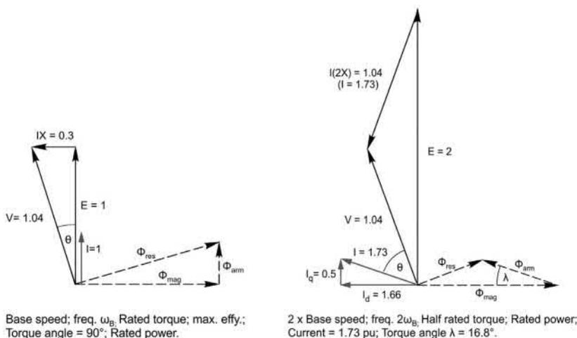
FIG. 9.22 PM motor phasor diagram—field oriented control. Full rated torque at base speed (left), half rated torque at twice base speed (right).
