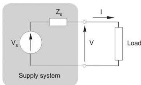
FIG. 6.1 Equivalent circuit of supply system.
