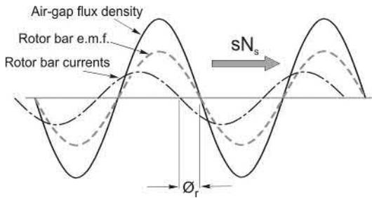
**FIG. 5.20** Pattern of air-gap flux density, induced e.m.f. and current in cage rotor bars at high values of slip (These waveforms should be compared with the corresponding ones when the slip is small, see Fig. 5.17).
