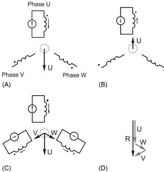
FIG. 8.1 Space phasor representation of m.m.f. waves.
