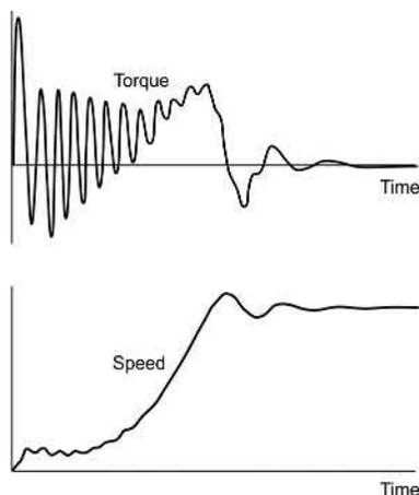
**FIG. 6.7** Run-up of unloaded motor, showing torque transients persisting for the first few cycles of the supply.
