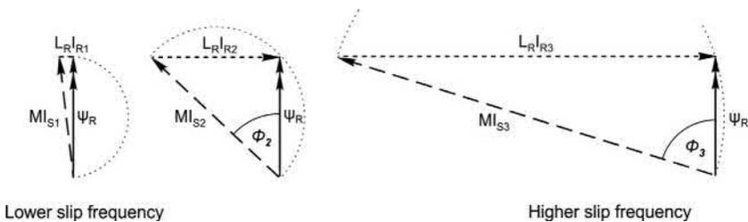
**FIG. 8.8** Constant rotor flux linkage space phasors at low, medium and high values of slip, showing variation of stator current required to keep rotor flux constant.
