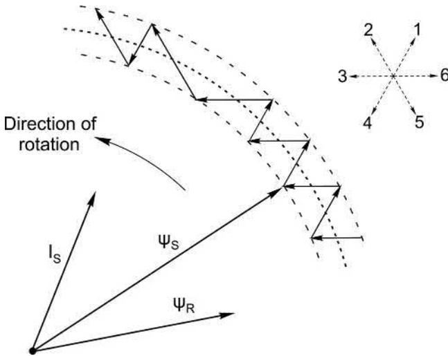
**FIG. 8.26** Trajectory of stator flux linkage under steady-state conditions.
