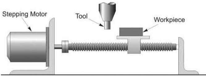
**FIG. 10.3** Application of stepping motor for open-loop position control.
