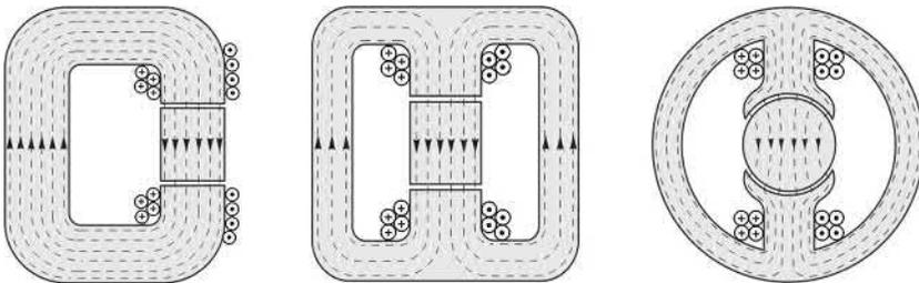
**FIG. 1.11** Evolution of d.c. motor magnetic circuit from gapped C-core.
