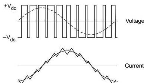
**FIG. 7.1** Typical voltage and current waveforms for PWM inverter-fed induction motor. (The fundamental-frequency component is shown by the dotted line.)
