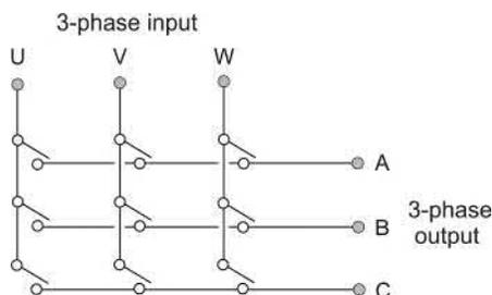
FIG. 2.29 Matrix converter power circuit.
