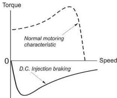
FIG. 6.20 Torque-speed curve for d.c. injection braking of cage motor.
