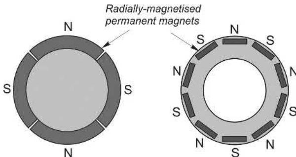
FIG. 9.3 Permanent magnet synchronous motor rotors; 4-pole (left); 10-pole (right).
