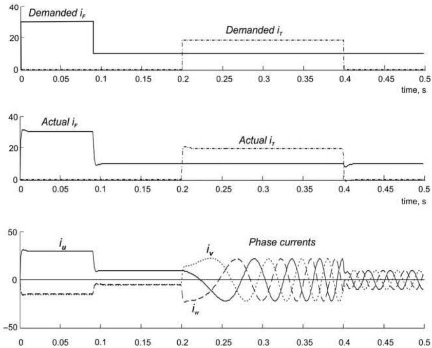
**FIG. 8.22** Experimental results showing build-up of flux followed by sudden demand for step increase in torque until motor reaches its target speed. (Courtesy of Nidec—Control Techniques.)
