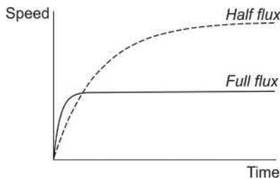
**FIG. 1.18** Effect of flux density on the acceleration and steady running speed of primitive d.c. motor with no mechanical load.
