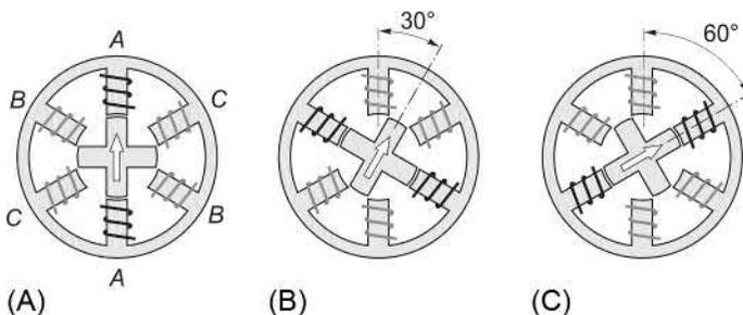
**FIG. 10.5** Principle of operation of  $30^\circ/\text{step}$  variable-reluctance stepping motor.
