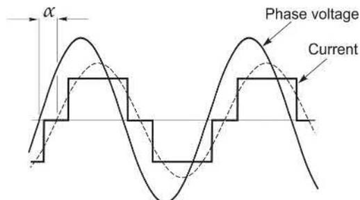
FIG. 4.10 Supply voltage and current waveforms for single-phase converter-fed d.c. motor drive.
