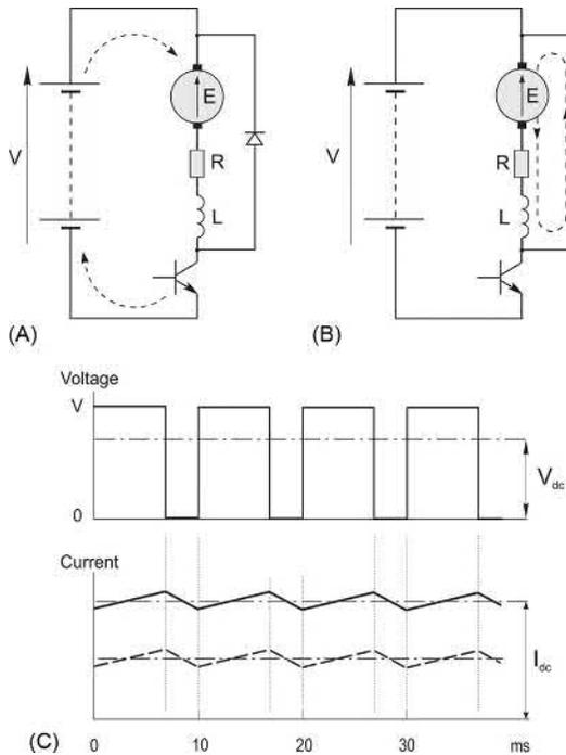
**FIG. 4.14** Chopper-fed d.c. motor. In (A) the transistor is ‘ON’ and armature current is flowing through the voltage source; in (B) the transistor is ‘OFF’ and the armature current freewheels through the diode. Typical armature voltage and current waveforms are shown at (C), with the dotted line representing the current waveform when the load torque is reduced by half.
