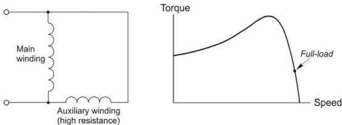
FIG. 6.25 Single-phase split-phase induction motor.
