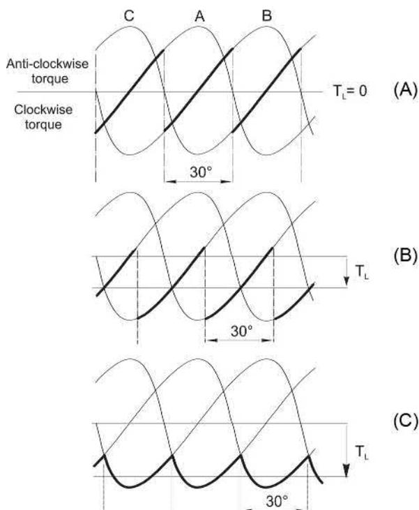
**FIG. 10.13** Static torque curves indicating how the average steady-state torque ( $T_L$ ) is developed during constant-frequency operation.
