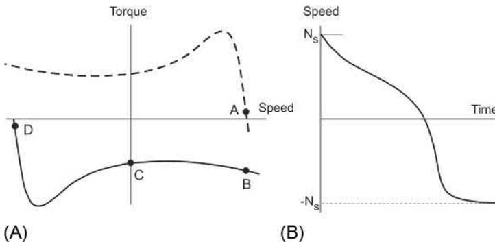
FIG. 6.19 Torque-speed and speed-time curves for plug reversal of cage motor.
