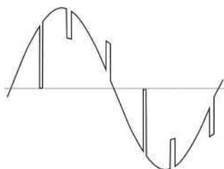
**FIG. 4.11** Distortion of line voltage waveform caused by overlap in three-phase fully-controlled converter. (The width of the notches has been exaggerated for the sake of clarity.)
