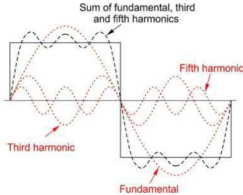
FIG. 2.16 Harmonic components of a square wave.
