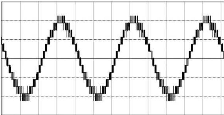
FIG. 2.24 A 13-level inverter voltage waveform.
