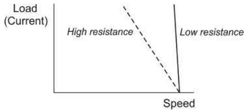
**FIG. 1.19** Influence of resistance on the ability of the motor to maintain speed when load is applied.
