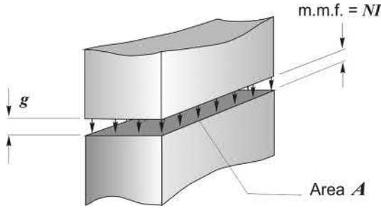
FIG. 1.9 Air-gap region, with m.m.f. acting cross opposing pole-faces.
