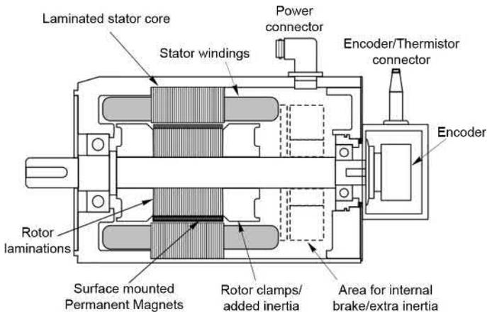
**FIG. 9.33** Typical high inertia permanent magnet synchronous motor. (Courtesy Nidec—Control Techniques Dynamics Ltd.)
