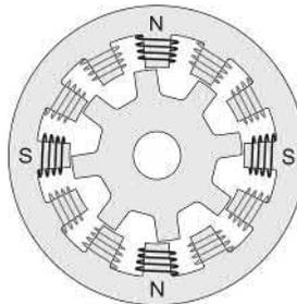
**FIG. 10.23** Typical switched reluctance motor. Each of the twelve stator poles carries a concentrated winding, while the eight-pole rotor has no windings or magnets.
