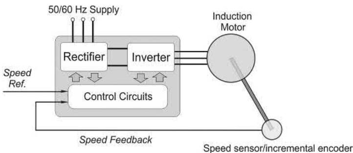
**FIG. 7.2** General arrangement of inverter-fed variable-frequency induction motor controlled-speed drive.
