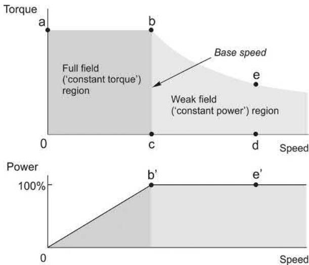
FIG. 3.10 Regions of continuous operation in the torque-speed and power-speed planes.
