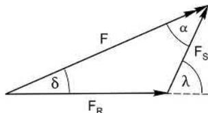
**FIG. 9.6** Space phasors showing rotor, stator, and resultant m.m.f.’s.
