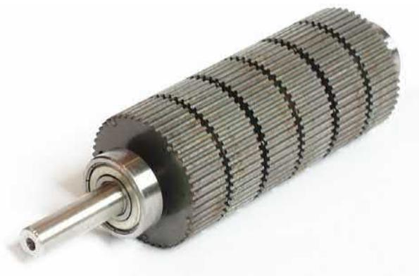
**FIG. 10.7** Rotor of size 34 (3.4 in. or 8 cm diameter) 3-stack hybrid 1.8° stepping motor. The dimensions of the rotor end-caps and the associated axially-magnetised permanent magnet are optimised for the single-stack version. Extra torque is obtained by adding a second or third stack, the stator simply being stretched to accommodate the longer rotor. (*Courtesy of Astrosyn International Technology Ltd.*)
