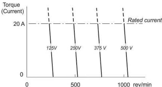
FIG. 3.9 Family of steady-state torque-speed curves for a range of armature voltages.
