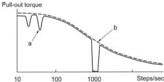
**FIG. 10.20** Pull-out torque–speed curves for a hybrid stepping motor showing (curve a) low-speed resonance dips and mid-frequency instability at around 1000steps/s; and improvement brought about by fitting an inertial damper (curve b).
