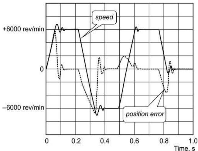
FIG. 9.35 Permanent magnet motor drive performance under rapid reversal test.
