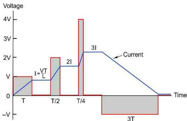
FIG. 8.10 Current (blue) when step voltages (red) are applied to a pure inductor.
