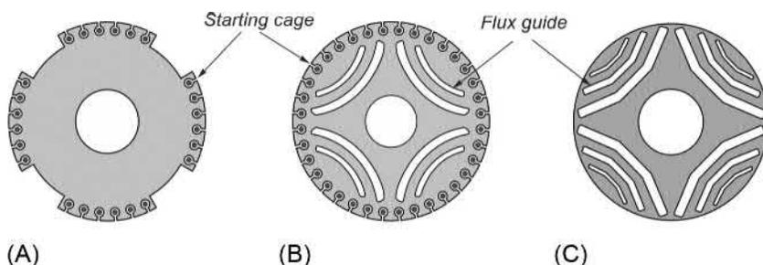
FIG. 9.4 Reluctance motor rotors (4-pole).
