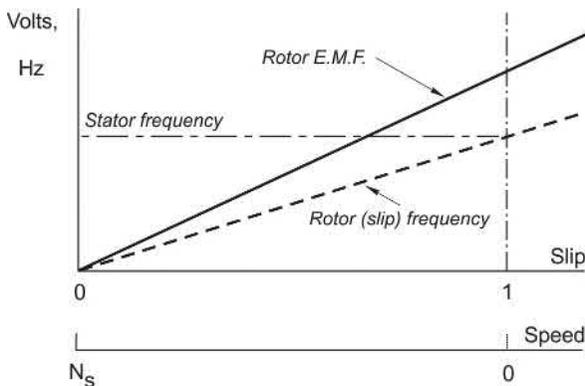
FIG. 5.14 Variation of rotor induced e.m.f. and frequency with speed and slip.
