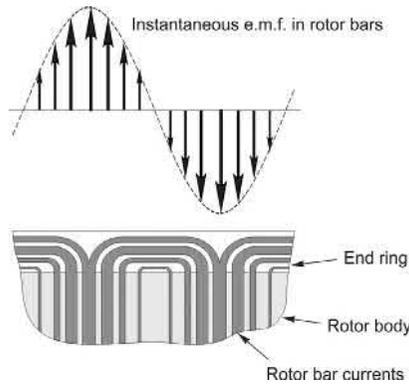
FIG. 5.16 Instantaneous sinusoidal pattern of rotor currents in rotor bars and end-rings. Only one pole-pitch is shown, but the pattern is repeated.
