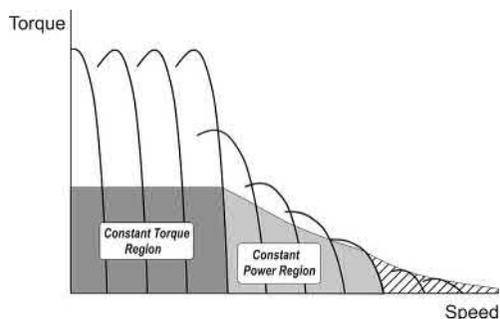
**FIG. 7.5** Constant torque, constant power, and high-speed motoring regions.
