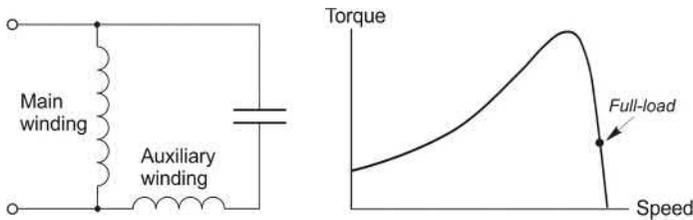
FIG. 6.24 Single-phase capacitor-run induction motor.
