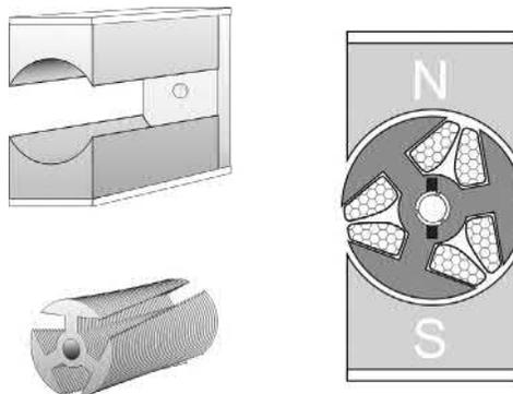
FIG. 3.17 Miniature d.c. motor for use in models and toys.
