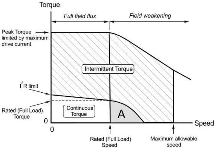
**FIG. 9.36** Limits of operation of a typical brushless PM motor.
