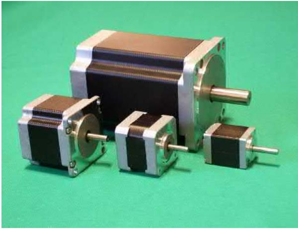
**FIG. 10.8** Hybrid 1.8° stepping motors, of sizes 34 (3.4 in. diameter), 23 and 17 and 11. (Courtesy of Astrosyn International Technology Ltd.)
