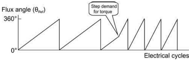
**FIG. 8.21** Flux angle reference showing response to a sudden step demand for increased torque.
