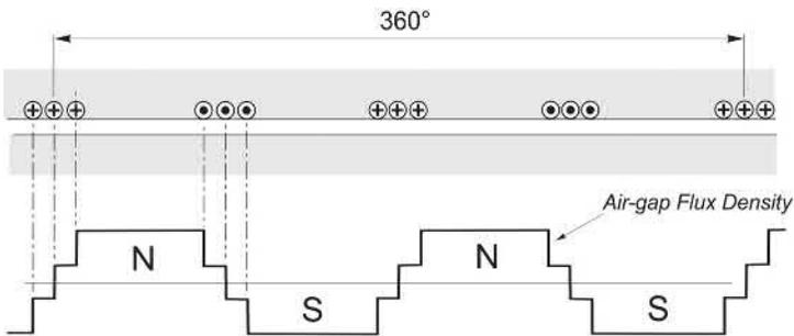
**FIG. 5.4** Developed diagram showing flux density produced by one phase of a single-layer winding having three slots per pole per phase.
