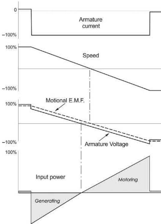
**FIG. 3.13** Regenerative reversal of d.c. motor from full-speed forward to full-speed reverse, at maximum allowable torque (current).
