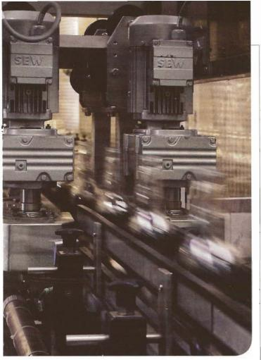
The SEW-Eurodrive DRP NEMA Premium motor visible in this recycling application is noteworthy in that its internal construction is optimized to handle numerous stop-starts for applications characterized by 1,000 to 2,000 cycles per hour. It is also the only premium-efficient motor with built-in encoder and an integral brake.
