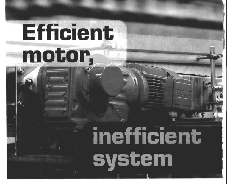
Other elements in the drivetrain can swamp out the effects of super-efficient induction motors.
