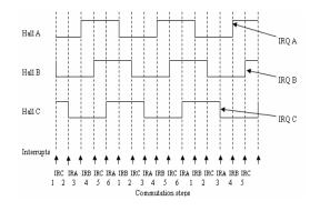
Figure 9. Output of Hall-Effect Sensors
