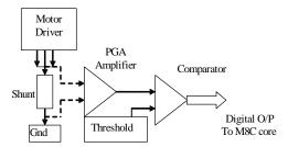
Figure 11. Current Measurement
