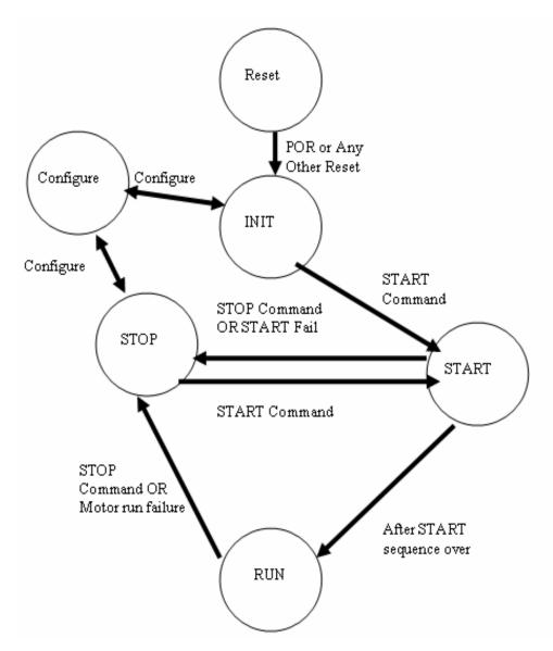
Figure 20. Motor Control State Machine
