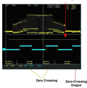
Figure 8. Back EMF Zero-Crossing Detection, Zero-Crossing Signals
