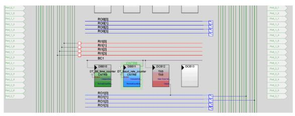
Figure 15. PSoC Designer Digital Blocks used for LIN Master Data Reception Configuration
