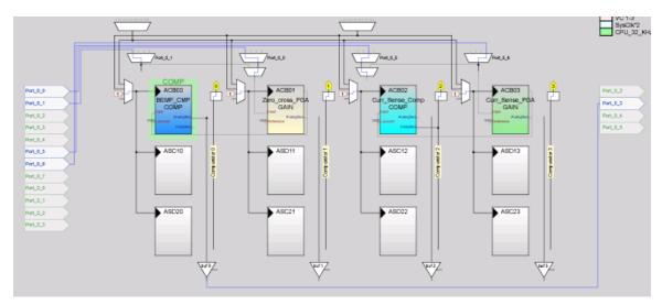
Figure 16. PSoC Designer Analog Blocks used for LIN Slave and BLDC Motor Controller
