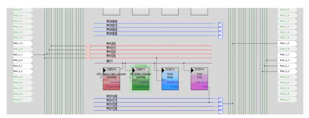
Figure 14. PSoC Designer Digital Blocks used for LIN Slave Data Reception Configuration
