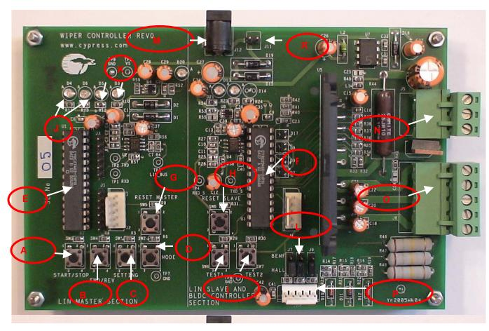
Figure 21. PSoC Automotive Motor Control BLDC Board
