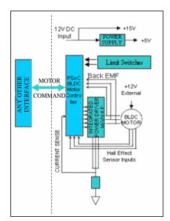
Figure 17. PSoC Automotive BLDC Interfacing to Other Systems
