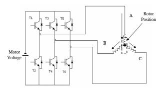
Figure 10. Alignment Phase Triple Half Bridge
