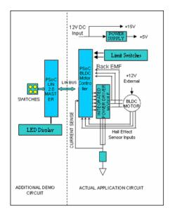
Figure 12. PSoC Automotive BLDC Block Diagram
