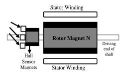
Figure 1. BLDC Motor Transverse Section
