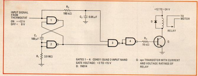
1. Restart delay. Motor is held off for a minimum time given by  $R_1C_1$  in this circuit arrangement. NAND-gate one-shot multivibrator starts delay pulse when thermostat goes off, so delay is not added to thermostat off-time. Quad NAND gate keeps component count low, and npn transistor allows flexibility in gate voltages. The time constant of  $C_2$  and  $R_2$  smooths over any contact bounce in the actuating relay.
