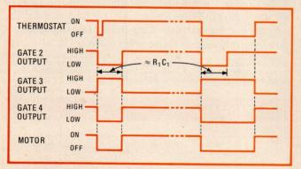
**2. Timing.** When thermostat goes off, gate 2 goes low and motor goes off. Motor then stays off until both thermostat and gate 2 are high again; gate 2 stays low for time of approximately  $R_1C_1$ , so motor is off for at least that long, and longer if thermostat is off longer.
