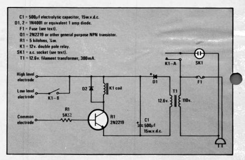
high level is reached and stays on until the pump removes enough water to reach the low level. Then it shuts off and doesn't cycle on until the water level is once again high. This difference between turn-on and turn-off is called *hysteresis* and can be adjusted by simply increasing or decreasing the height of the two electrodes.
