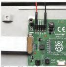
The 15-way DSI cable is plugged into its socket on the driver PCB with its contacts facing up. This close-up view also shows the 5V supply output leads which run to pins 2 & 6 on the RPi's GPIO header.
