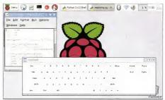
The virtual keyboard can be resized and can also be configured so that it always sits on top of other open windows (just click the keyboard symbol at top left of its window and select Layer -> Always On Top).
