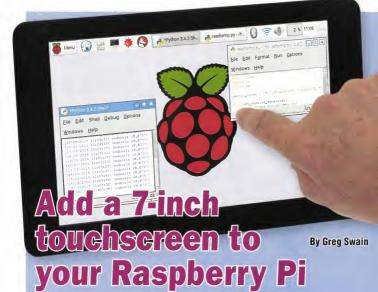
If you want to turn your Raspberry Pi (RPi) into a completely self-contained unit, then this 7-inch (18cm) Touchscreen Display is the answer. It's a cinch to hook-up and get going, has a bright 800 x 480 pixel display and includes a mounting kit so that you can attach the RPi module to the display's metal back-plate.
