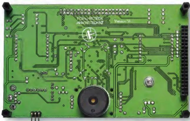
The piezo buzzer and the 40-way connector for the LCD panel mount on the rear of the PCB. The connector plugs directly into a matching pin header on the back of the 5-inch LCD panel (see photos and page 71, August 2016).
