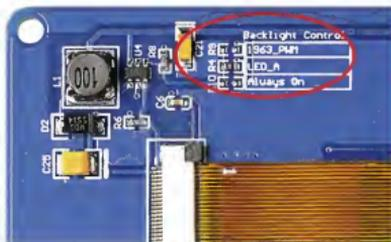
As explained in the text, if you move the 0Ω resistor from position "LED\_A" to "1963\_PWM" you will be able to control the display's brightness in 1% steps. This photograph shows the back of a 5-inch display but the other display sizes each have a similar set of jumper positions.
