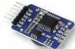
This is the RTC module that the Explore 100 is designed to use. It employs the Maxim/Dallas DS3231 which can keep the time to better than  $\pm 2$ ppm and its battery back-up facility will retain the time during power outages. Note that the existing pin header has to be removed and two straight pin headers soldered to the underside of the PCB at both ends of the module.
