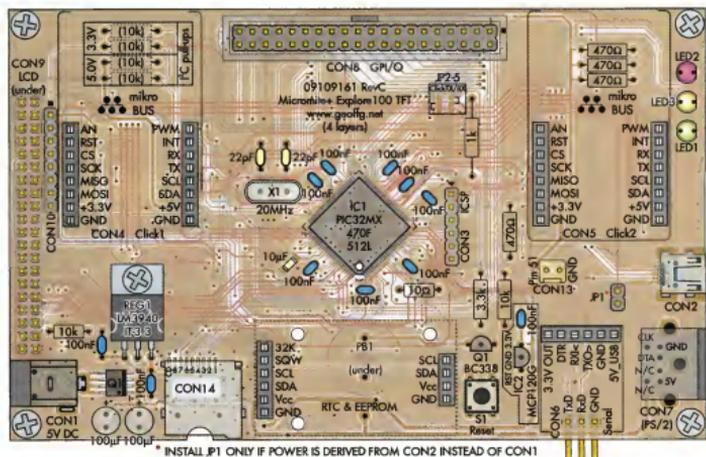
Fig 2: follow this parts layout diagram to build the PCB. The Explore 100 uses mostly through-hole components, with just five surface-mount parts (including the PIC32 micro). CON1 can be either a 2.1mm DC power connector or a micro-USB socket (the SILICON CHIP version of the PCB accepts both). Note that the SILICON CHIP PCB also includes a micro-SD card socket (CON14), whereas the original PCB simply includes a header for connecting the card socket (CON10).
