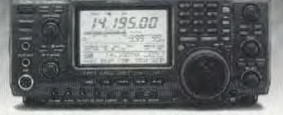
The IC-746 Pro covers 160-10 meters plus 6 and 2 meters with 100 watts on all bands. Call or visit our website for further details and pricing on this and other ICOM radios.
