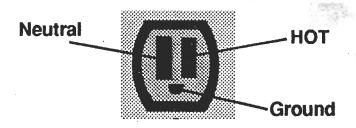
The hot slot is the one charged with electricity. The voltage in this slot oscillates back and forth between +170 and -170 volts.
