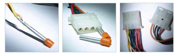
a click sound heard after you have overcome the pressure. Exactly as this click is heard you need to remove the wire in question, with its pin, from behind out of the plastic housing. If this doesn't work exactly as desired, it can help to twist the sleeve around while you are pulling.
