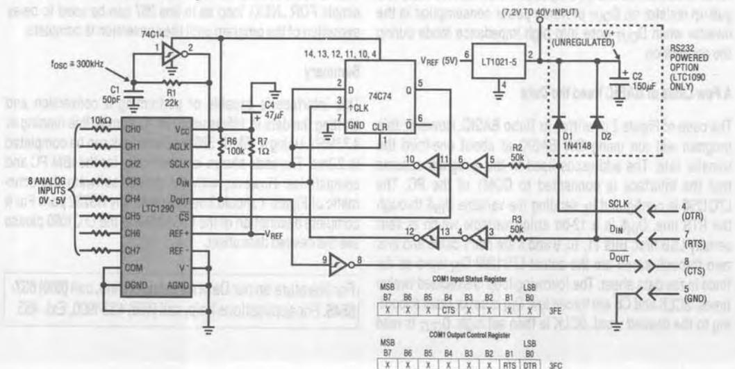
Figure 1. LTC1290 to IBM PC Serial Port Interface
