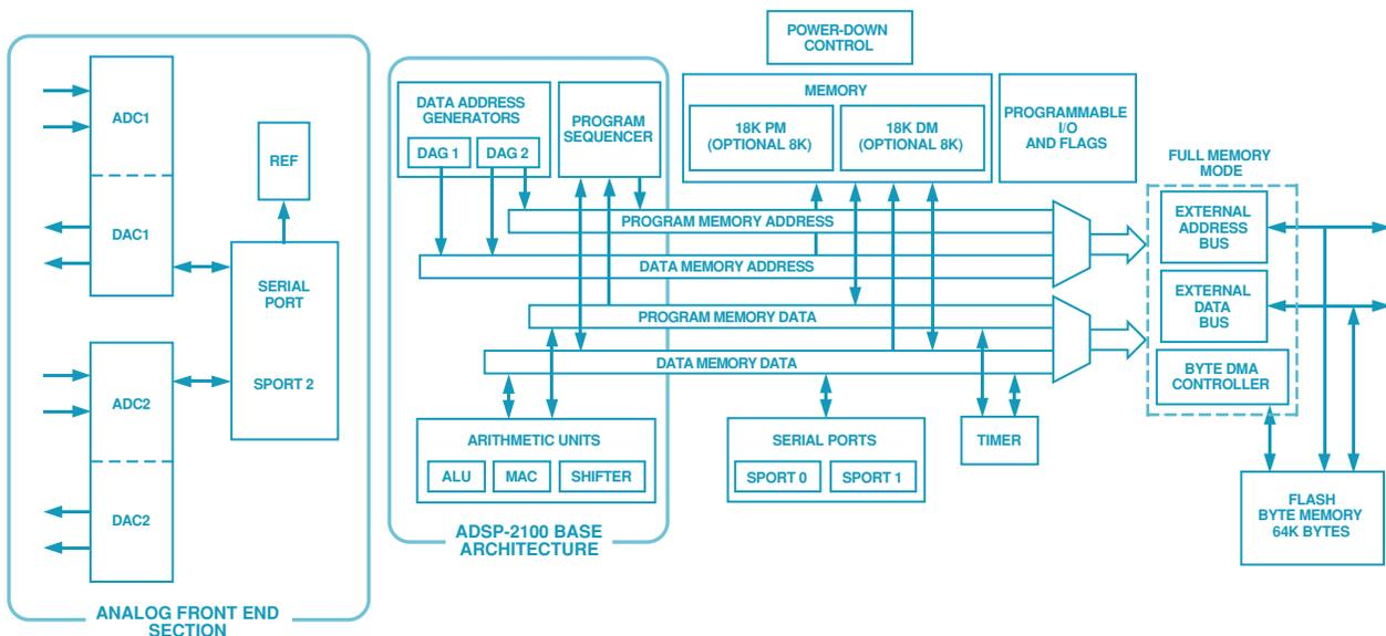
Figure 5. AD73522 dspConverter.
