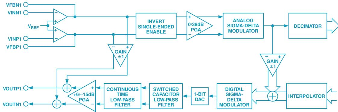
Figure 6. Analog front-end subsection of the AD73522 dspConverter.
