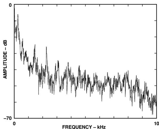
Figure 1. Profile of server fan noise.
