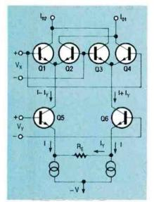
FIG. 7—FOUR-QUADRANT MONO-LITHIC modulator is basically two twoquadrant transconductance multipliers.
