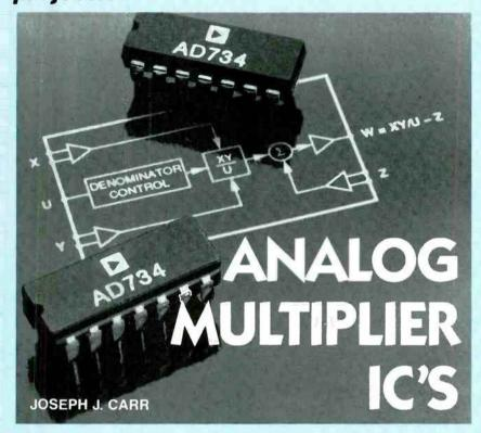
MONOLITHIC ANALOG MULTIPLIERS can multiply, divide, square, and extract the square root of analog inputs that represent various arithmetical values. Multiplier IC's can accept one or two inputs, and calculate analog outputs with few external components. These analog "math blocks" play important roles in data acquisition, automatic control, and instrumentation circuits. It's all a matter of how the input signals are connected to the multiplier.
