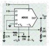
FIG. 12-SCHEMATIC DIAGRAM of the AD532 organized as a divider.
