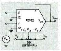
FIG. 13—SCHEMATIC DIAGRAM of the AD532 organized as a squarer.
