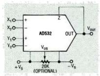
FIG. 11-SCHEMATIC DIAGRAM of the AD532 organized as a multiplier.
