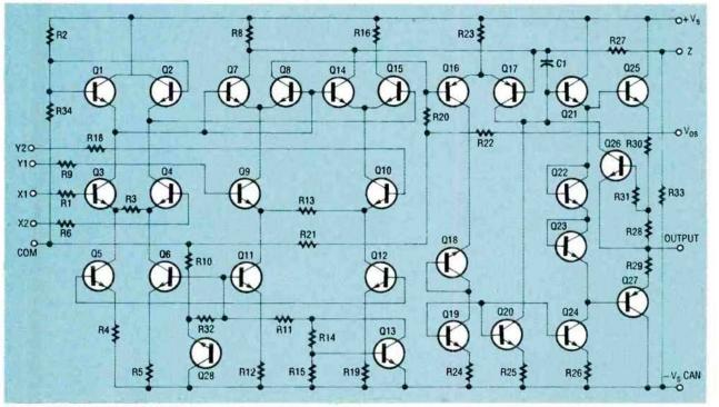
FIG. 9—SCHEMATIC DIAGRAM for a monolithic AD 532 multiplier.
