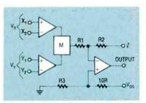
FIG. 8—FUNCTIONAL BLOCK DIAGRAM of an Analog Devices AD532 showing its differential inputs. Note the single Z input and the  $V_{\rm os}$  input.
