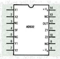
FIG. 10-PINOUT DIAGRAM for an AD532 in a 14-pin DIP.
