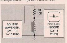
FIG. 3—USE THIS SET UP to perform a ringing test on a coil or transformer. The waveform displayed depends on the transformer's inductance and capacitance.
