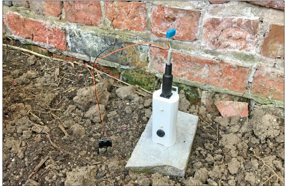
Figure 6. GoNotify busy monitoring air humidity and temperature and soil humidity in a greenhouse.
