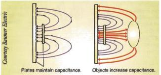
As objects enter a capacitive sensor's detection zone, capacitance increases; circuit natural frequency shifts towards an oscillation frequency, causing amplitude gain.
