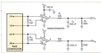
Figure 2 At the terminal, IC<sub>4</sub> converts the signals it receives from the interface to LVTTL levels and then feeds them to a set of passive filters.
