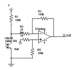
The reference source can easily be created with a potentiometer. Starting with this basic design we should be able to create an acceptable "black box" for the flame detection. We can narrow the field of view by placing the phototransistor inside a tube, and we can enhance its sensitivity by using a reflector. Experimentation will be necessary. Let me know of any improvements you make so we can post them on this site.
