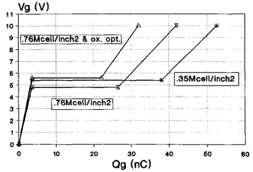
Fig. 7 - Oxide and layout influence on gate charge.
