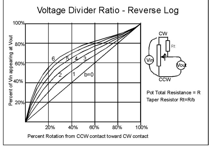
There are two ways to hook up a pot. You can hook it up as a three terminal voltage divider as we've seen above, or as a variable resistance, the two-terminal connection (sometimes called a rheostat connection for historical reasons).
