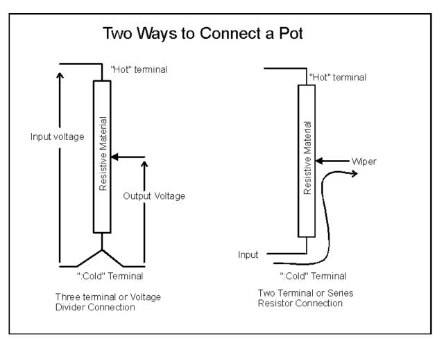
In the two terminal connection, the resistance through the pot is what we're interested in, not the voltage divider ratio.
