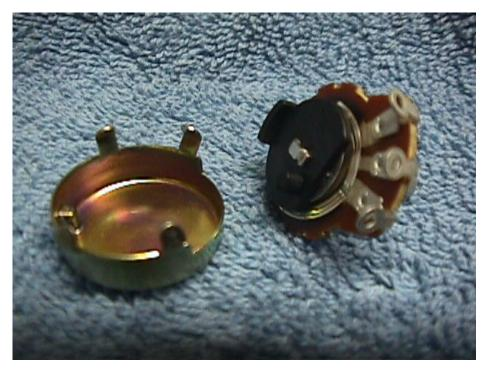
All the fun stuff appears to be inaccessible under that black plastic cover. Actually, that cover performs a couple of very useful functions; it serves to hold the wiper in place, and also interacts with the stop on the case to set the mechanical rotation limits. If you remove the tab on the plastic disk and reassemble the pot, it will now rotate freely 360 degrees. Here's a little better view of the shaft/wafer/wiper assembly.
