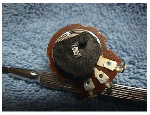
Looking closely, you can see that the shaft is held onto the plastic disk by being mechanically squashed into place. That is quick, and makes for cheap pots, but it can't be removed and successfully reassembled. That is a peculiarity of this brand, as some pots can be disassembled and reassembled successfully. In the next picture, I've used a big pair of diagonal cutters to remove the plastic disk and the metal wipers. This exposes the bare conductor assembly.
