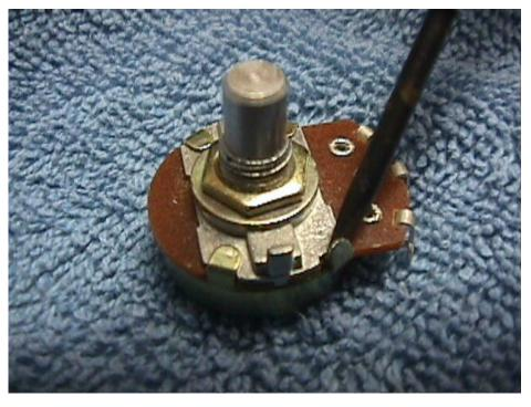
When they're all bent up, you can lift the shaft and phenolic wafer assembly out of the back housing like this.
